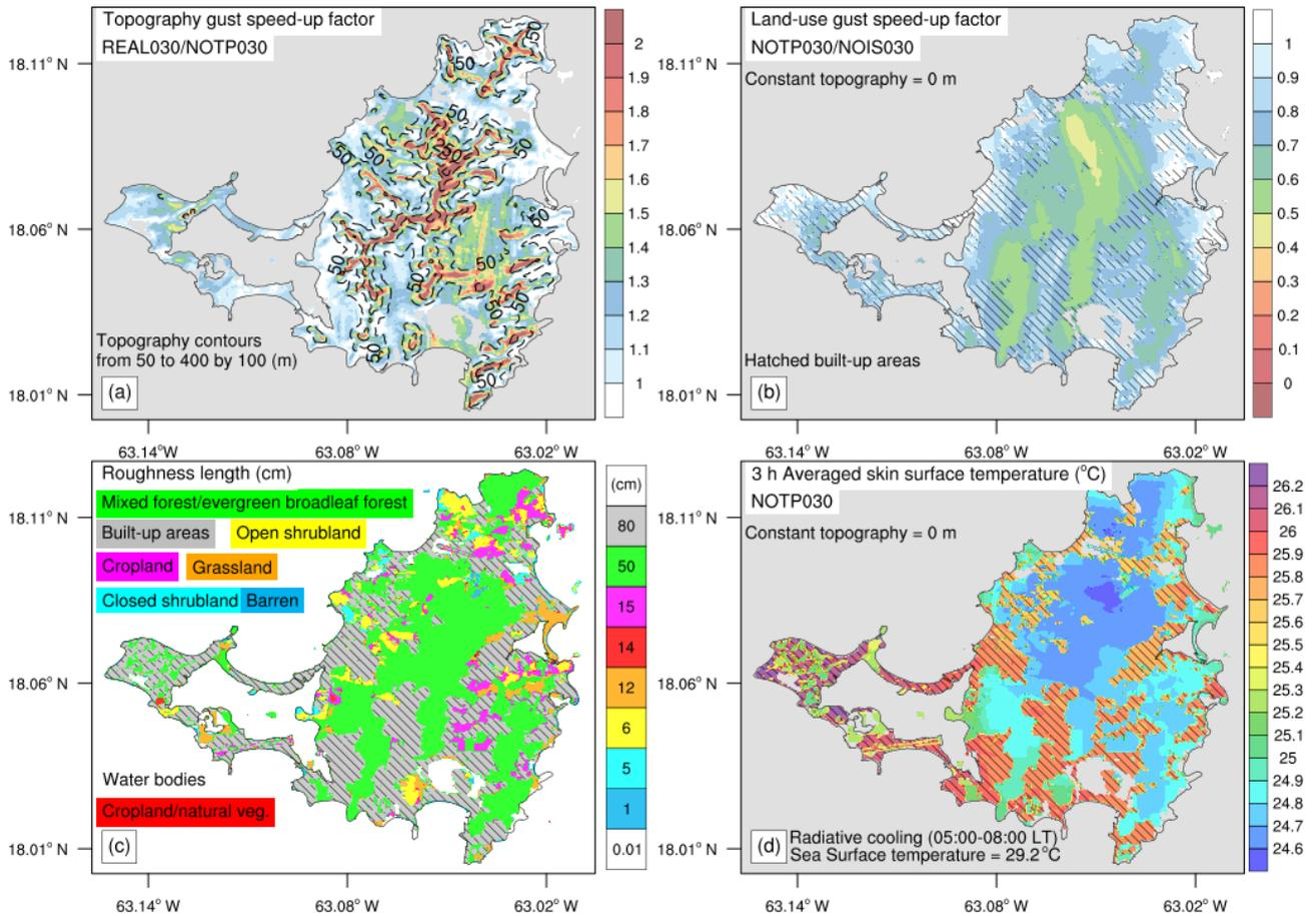
**Figure 12.** Effects of Saint Martin island terrain on maximum instantaneous gust. (a) Topography gust speed-up factor. (b) Land-use gust speed-up factor. (c) Surface roughness length (cm). (d) 3 h averaged skin surface temperature during the landfall in °C: non-topography experiment, NOTP030.
