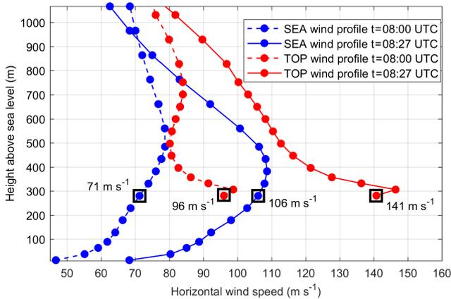
**Figure 10.** Vertical profile of the REAL030 instantaneous horizontal wind speed ( $\text{m s}^{-1}$ ) at 08:00 UTC and at the peak gust time 08:27 UTC: comparison between the upstream winds over the sea (SEA) and the orographic winds over the mountain top (TOP).
