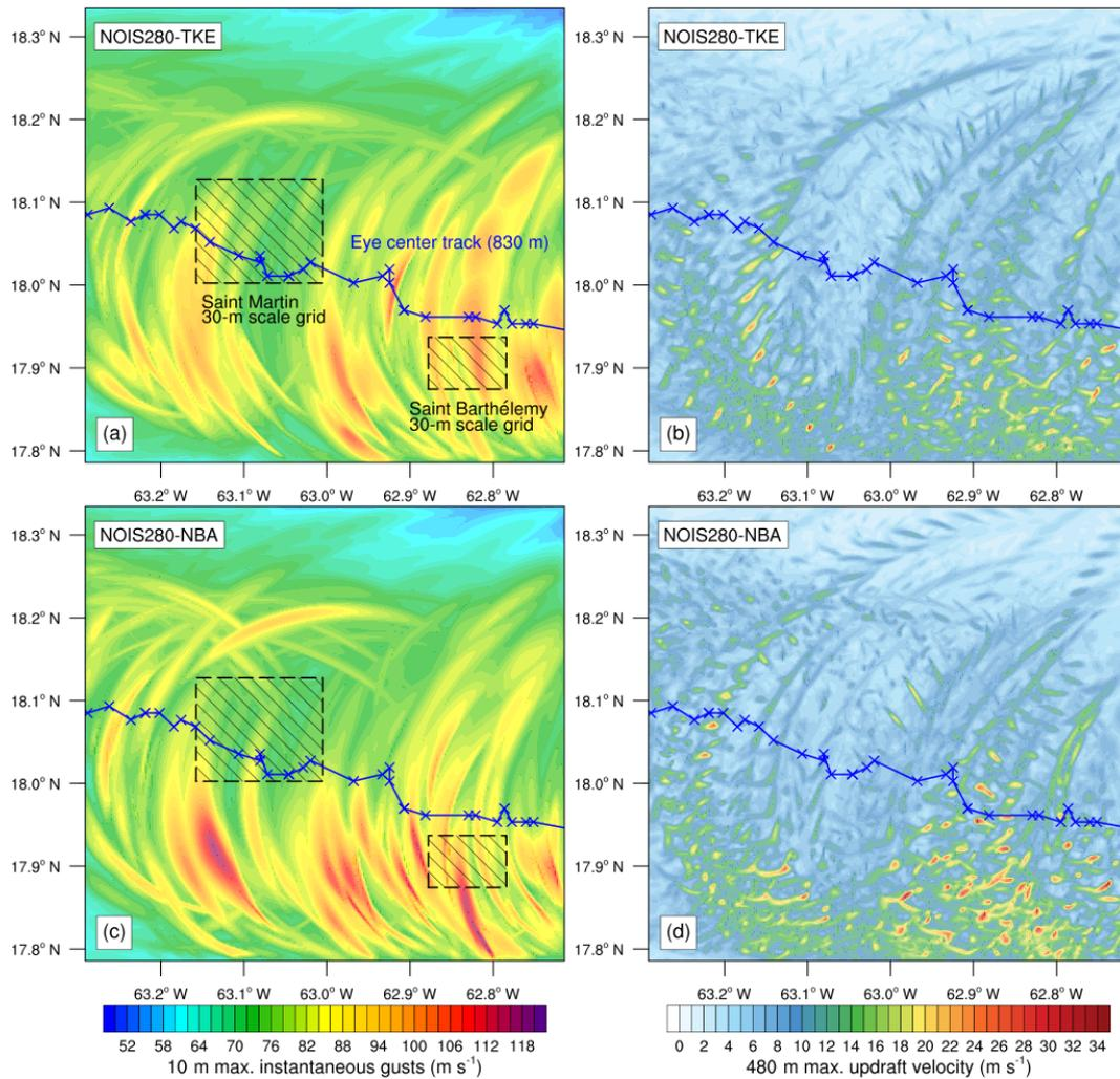
**Figure 4.** Comparison between the TKE SFS scheme and the NBA SFS scheme at 280 m scale: non-island experiment NOIS280. **(a, c)** Maximum instantaneous gusts ( $\text{m s}^{-1}$ ) occurring at 10 m during the 6 h of simulation (history output interval of 1 min). **(b, d)** Maximum updraft velocity ( $\text{m s}^{-1}$ ) occurring at 480 m during the 6 h of simulation.
