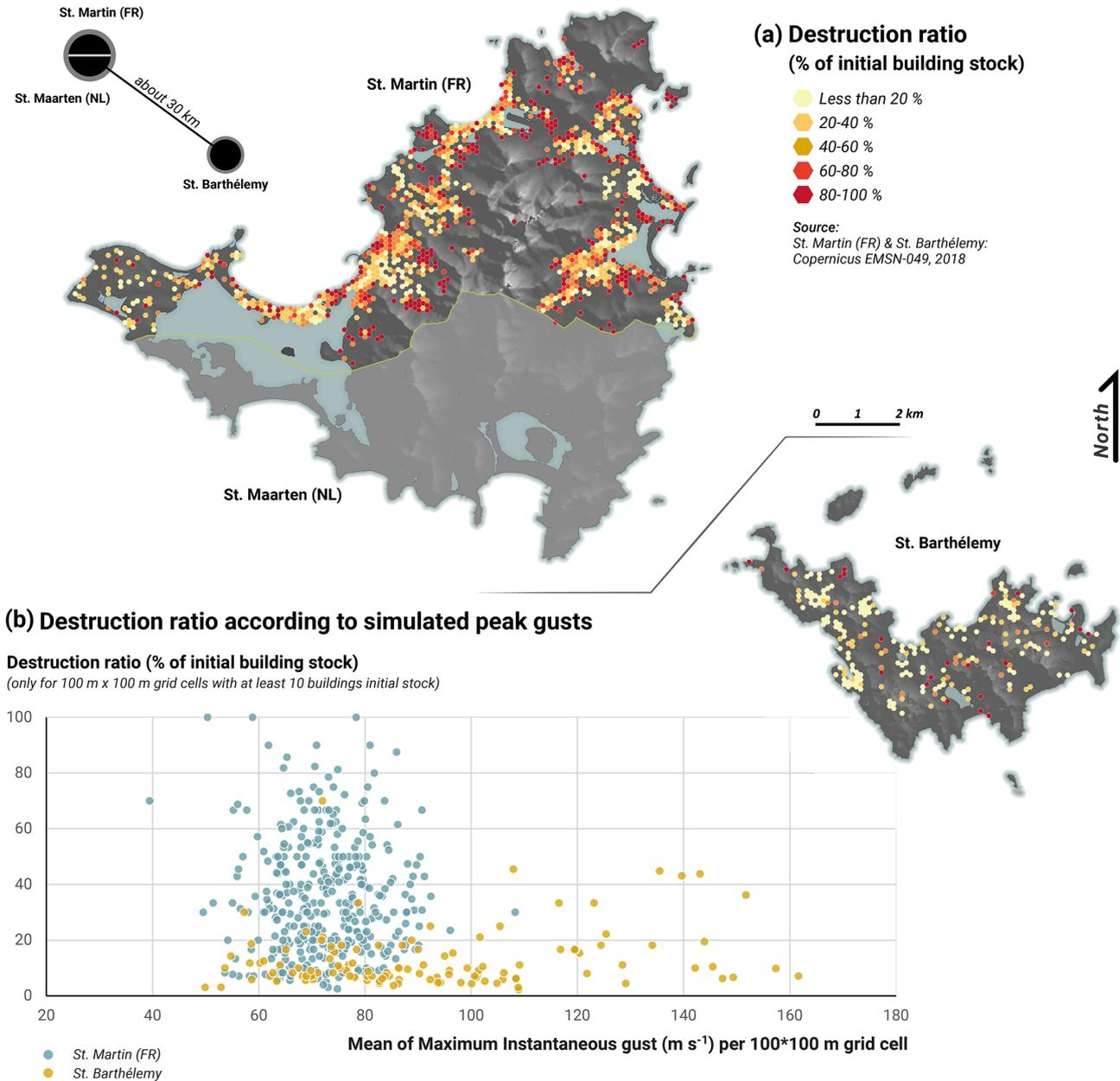
**Figure 13.** Analysis of relationships between Copernicus EMSN049 remote sensing damage map and simulated peak gusts (REAL030). **(a)** Destruction ratio map over Saint Martin (French entity, FR) and Saint Barthélemy (%). **(b)** Comparison with simulated maximum gusts ( $\text{m s}^{-1}$ ).
