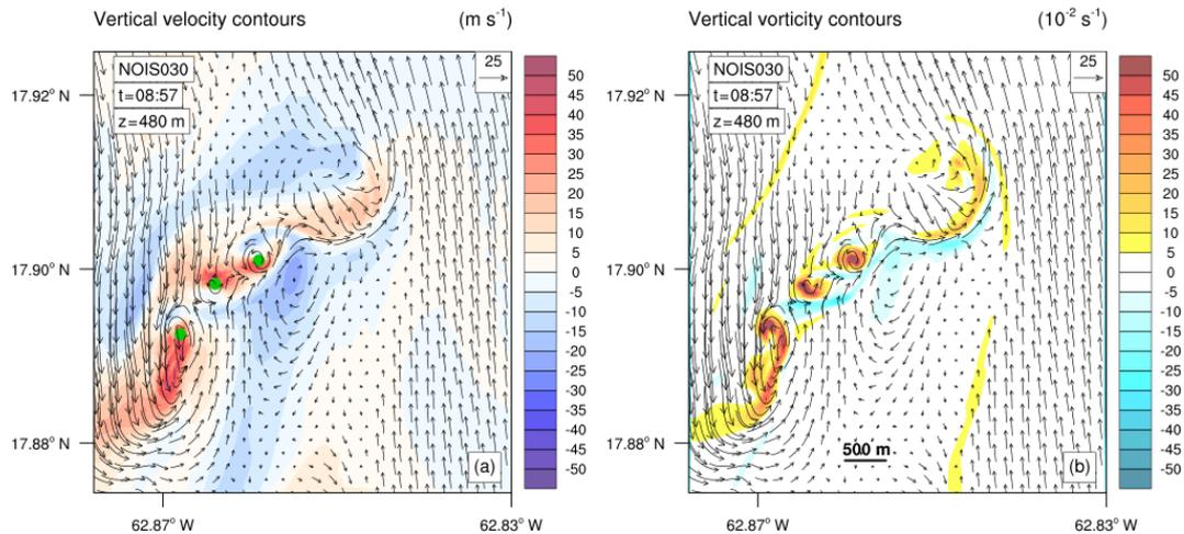
**Figure 6.** Tornado-scale vortices at 480 m level linked with the maximum simulated gust occurring at 08:57 UTC in NOIS030 dashed area (Fig. 4). (a) Perturbation vertical velocity contours ( $\text{m s}^{-1}$ ). (b) Vertical vorticity contours ( $10^{-2} \text{ s}^{-1}$ ). Perturbation horizontal wind vectors are plotted in the two panels.
