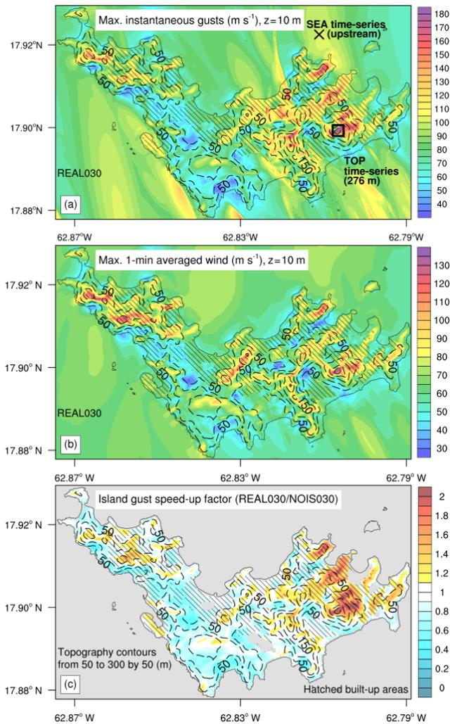
**Figure 8.** Saint Barthélemy 30 m scale maximum surface winds during the 6 h of simulation (history output interval of 1 min). (a) Maximum instantaneous gust ( $\text{ms}^{-1}$ ) with locations of two numerical time-series stations: SEA and TOP. (b) Maximum 1 min averaged wind in  $\text{ms}^{-1}$ . (c) Island gust speed-up factor (REAL030/NOIS030). Topography contours in meters and hatched built-up areas are plotted on the three panels.
