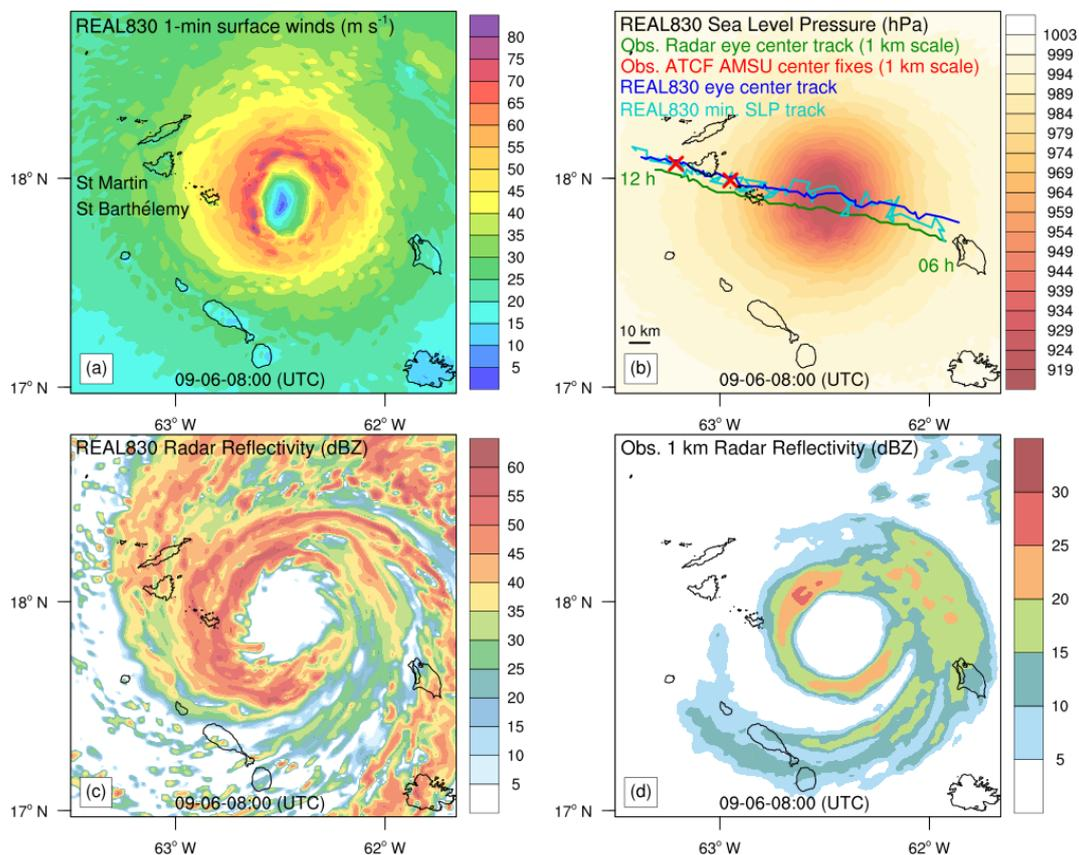
**Figure 3.** Simulated Irma eye at 830 m scale and at 08:00 UTC (REAL830). (a) Sustained surface winds ( $\text{m s}^{-1}$ ). (b) Sea level pressure (hPa) with simulated tracks and observed radar eye center track. The time interval for all tracks is 5 min. (c) Simulated radar reflectivity (dBZ). (d) Observed radar reflectivity (dBZ).
