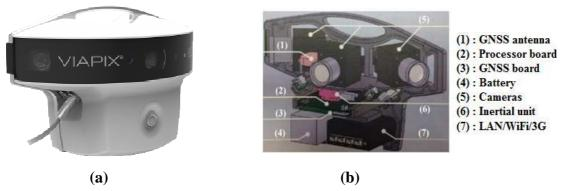
Figure 1 - (a) VIAPIX® Acquisition module, (b) Architecture.
