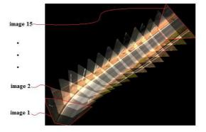
Figure 9 - The orthophoto obtained by merged images.
