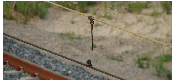
Figure 4. Dropper failure caused by fatigue.
