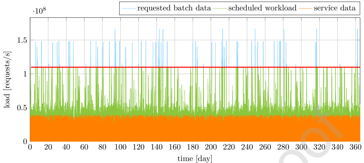
Figure 2: Example of the load (expressed as a histogram in number of requests per seconds) over time (in hours) which is executed after the IT sizing. The requests for services are in orange, the one for batches in blue. It results in the green processed requests using 1098 servers considering one year discretized into K = 8760 time slots of one hour and a flexibility of 3 hours.
