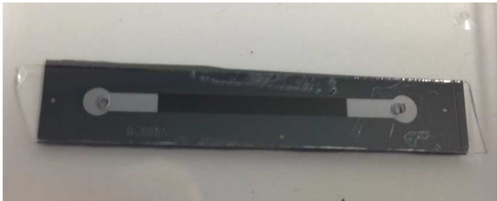
Fig. 1. (a) Schematic of a micro-channel with the micro structure region zoomed; (b) the picture of a Pyrex/Silicium/Pyrex sample
