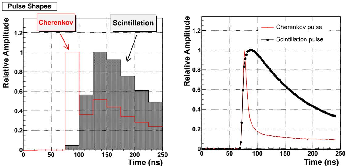
**Figure 4.** Left: comparison between the average pulse shape of a Ce-doped fiber (black) and an undoped fiber (red) using 80 GeV electrons. Right: average pulse shapes with better time granularity for Ce-doped fibers (black dots) and undoped fibers (red) obtained in previous test beam using an oscilloscope [8].
