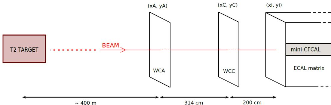
**Figure 2.** Sketch of the last stage of the H2 beam line at CERN, SPS. The ECAL matrix containing the mini-CFCAL is shown as well as the wire chambers WCA and WCC used in this analysis. The red arrow indicates the electrons beam direction.
