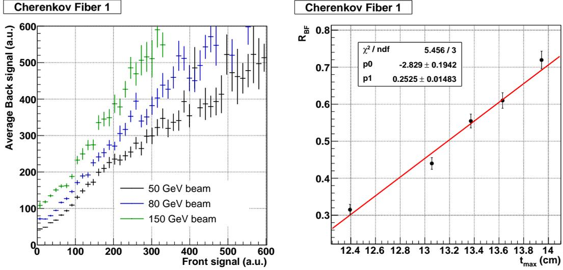
**Figure 8.** Left: the correlation between front  $F$  and back  $B$  signals of Cherenkov fiber number 1 is shown at different beam energy. Right: correlation between  $R_{BF}$  and the theoretical  $t_{\max}$  position for a given beam energy with a linear fit (red). Error bars represent the statistical uncertainty on the points.
