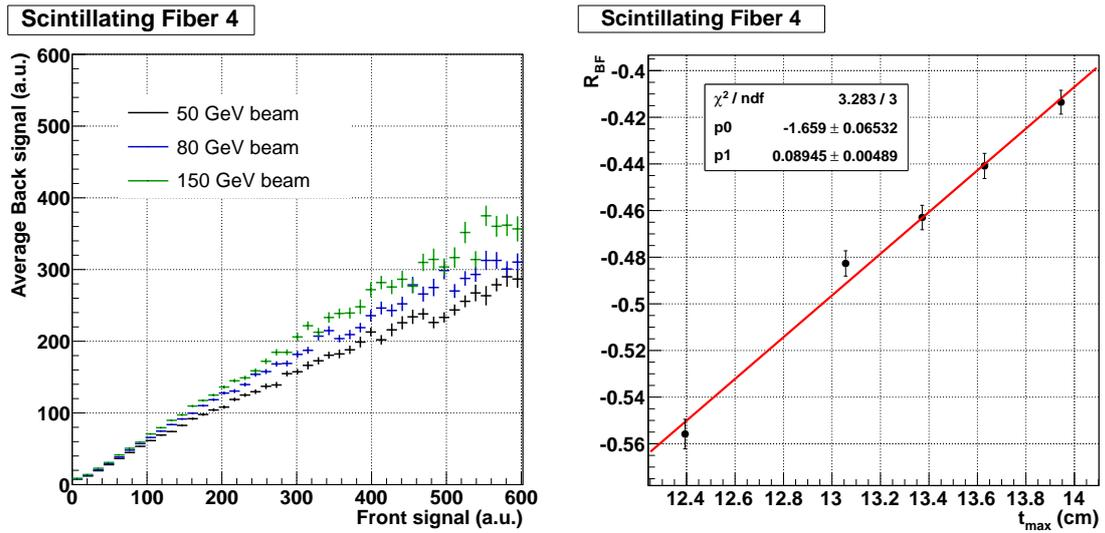
**Figure 9.** Left: the correlation between front  $F$  and back  $B$  signals of scintillating fiber number 4 is shown at different beam energy. Right: correlation between  $R_{BF}$  and the theoretical  $t_{\max}$  position for a given beam energy with a linear fit (red). Error bars represent the statistical uncertainty on the points.
