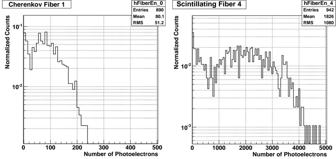
**Figure 5.** Distribution of photoelectrons measured from one end of a Cherenkov fiber (left) and a scintillating fiber (right) using 80 GeV electrons within a  $2 \times 2 \text{ mm}^2$  beamspot around the centre of the selected fiber.
