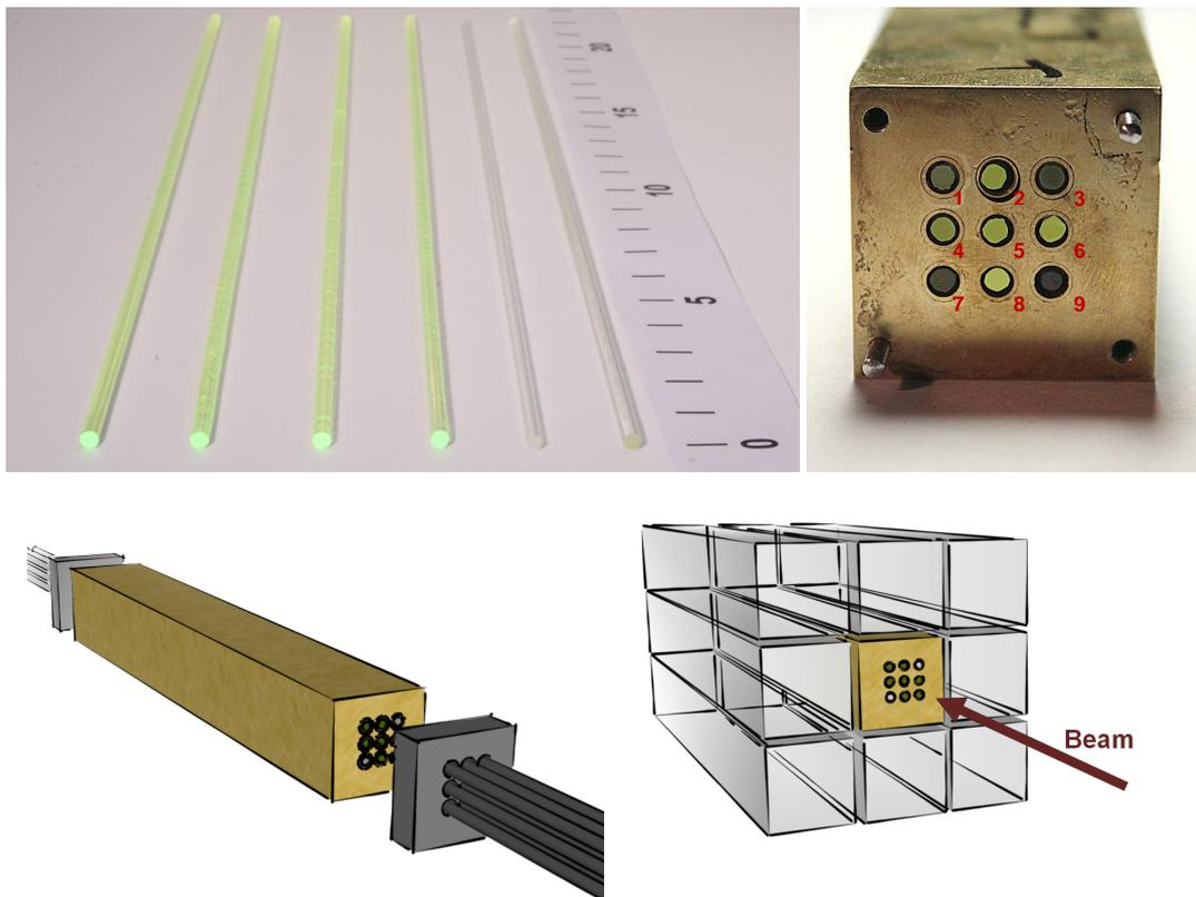
**Figure 1.** (Top) Pictures of a set of Cerium-doped (green color) and undoped (transparent) LuAG fibers and the brass absorber containing 9 LuAG fibers. (Bottom) The mini-CFCAL (brass absorber with 9 LuAG fibers) is connected to optical fibers for light extraction and inserted in a matrix of  $\text{PbWO}_4$  crystals.
