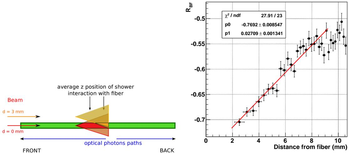
**Figure 10.** Left: a sketch to naively represent the drift of the average interaction point of the shower with a given a fiber when the electron impact point move away from the fiber centre. Right: correlation between the value of  $R_{BF}$  and the position the distance of electrons from the fiber. A linear fit is performed in the range (2,9) mm distance (red line). Error bars represent the statistical uncertainty on the points.
