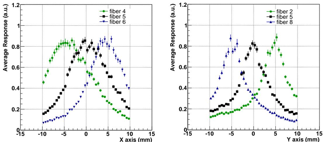
**Figure 6.** Left: average response of the fibers of the central row as a function impact point along the x axis: fiber 4 (green), fiber 5 (black), fiber 6 (blue). Right: average response of the fibers of the central line as a function impact point along the y axis: fiber 2 (blue), fiber 5 (black), fiber 8 (green).
