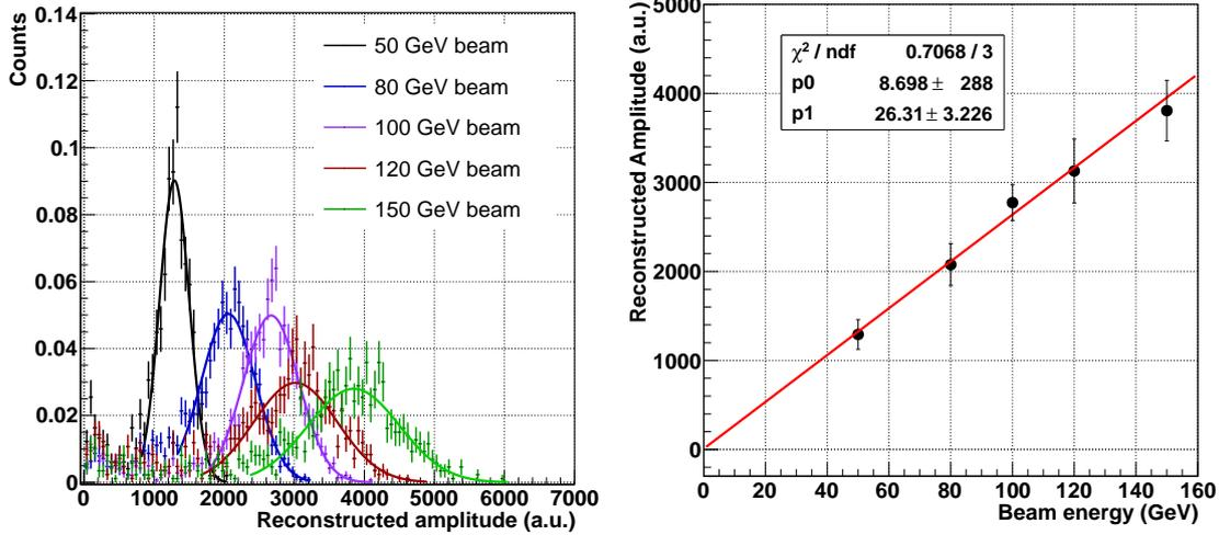
**Figure 7.** Left: distributions of reconstructed amplitude  $E_{\text{reco}}$  at different beam energy. Right: correlation between the peak value of  $E_{\text{reco}}$  distributions and the beam energy with a linear fit (red line). Error bars represent the statistical error on the estimation of peak position.
