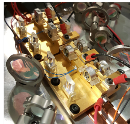
Fig. 1 (left) Simplified schematic of the experimental setup. (right) Photograph of the assembled CBC module.
