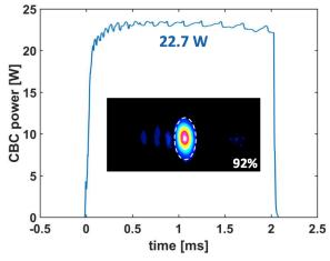
Fig. 3. Experimental pulse shape at the output of the CBC interferometer at 14.5 A in the tapered sections (average over 1 mn). (inset) Waist of the combined beam and power content in the central lobe. Bias conditions:  $P_{\rm in}$  = 20 mW,  $I_{\rm rw}$  = 300-400 mA, T = 25°C,  $\Delta t_{\rm qcw}$  = 2 ms, 10 % duty cycle
