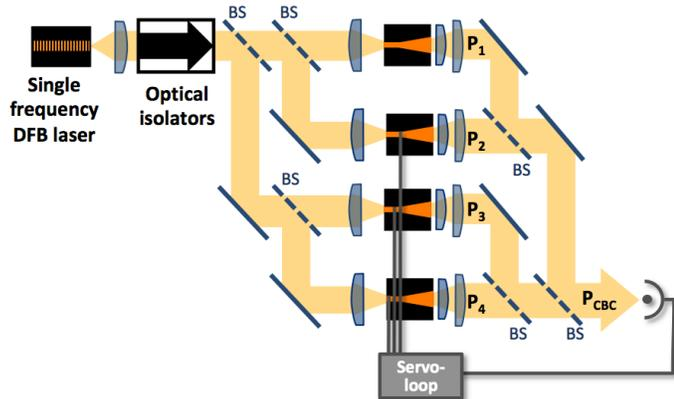
Fig. 2. Experimental setup of the CBC-interferometer with four high brightness tapered amplifiers. The amplified beams are collimated in SA and FA with a high NA aspheric lens ( $f = 2.35$  mm) and a cylindrical lens ( $f = 19$  mm). The phase correction is applied through the currents into the RWs.
