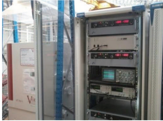
Fig. 3. Climatic chamber and power electronics as a test bench for the insulation materials.
