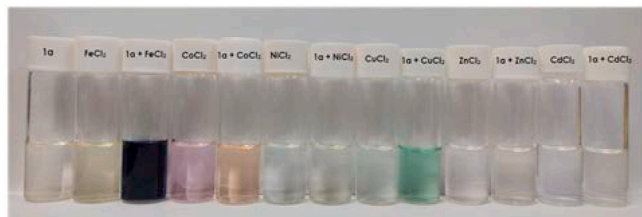
Fig. 4. Colorimetric behavior of compound 1a towards the addition of metal ions in methanol solutions.
