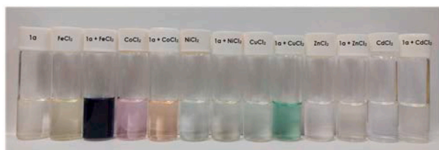
Fig. 4. Colorimetric behavior of compound 1a towards the addition of metal ions in methanol solutions.
