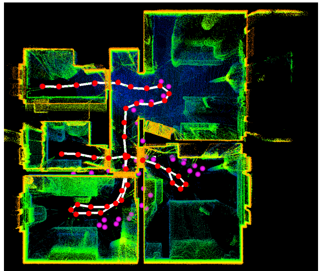
Fig. 6. 3D mapping of the Apartment sequence using the proposed method. The points of the map are colored regarding their height (blue being the lowest value, green in between and yellow the highest). In white the ground truth trajectory. In purple dots the trajectory computed with the plane-to-plane registration only. In red dots the trajectory computed with the full proposed NAP-ICP (combination of plane-to-plane and point-to-plane registration). Ceiling has been removed to ease visualization.
