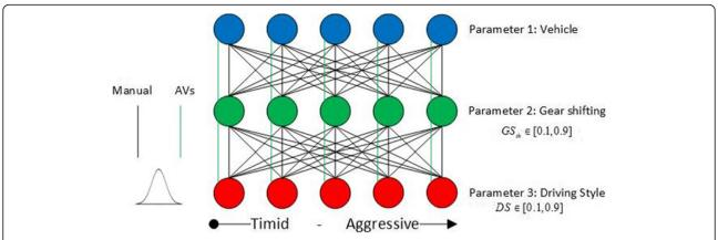
**Fig. 3** Creation of 125 individual driving profiles  $DP_i$  by choosing from a pool of 5 different cars, 5 gear shifting strategies and 5 driving styles. AVs are shown with green line and correspond to 5 individual profiles, one per each vehicle. The selection of the profiles during each simulation is performed based on a normal distribution around the average profile, i.e. the second value of each parameter
