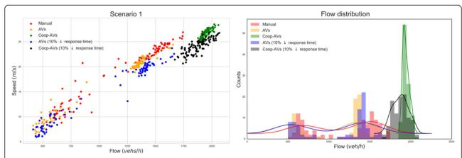
Fig. 4 a) Average speed and average flow values per vehicle type and simulation test run, b) Distribution of the average flow for the different test runs
