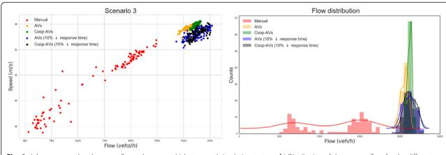
Fig. 6 a) Average speed and average flow values per vehicle type and simulation test run, b) Distribution of the average flow for the different test runs
