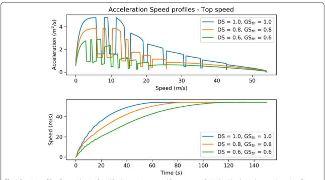
Fig. 1 Simulation of free-flow acceleration from 0 km/h to maximum speed for a commercial vehicle with a 9-speed automatic gearbox. Top: Acceleration-Speed profiles for three different drivers with different driving styles. Bottom: The simulated speed profiles for the same drivers
