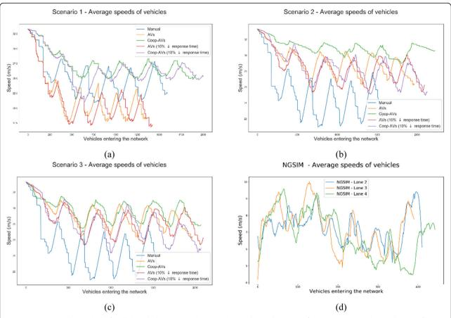
**Fig. 7** Average speed per vehicle, for all the vehicles entering the network. Sample simulation tests for Scenarios 1, 2 and 3 are shown in figures **a**), **b**) and **c**). Figure **d**) shows empirical observations in three lanes in a congested segment of the NGSIM database
