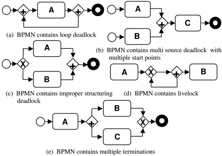
Figure 4. Structural errors in BPMN
