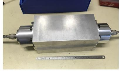
Fig. 15. a) Simulation of the corrugated waveguide in between the CWT and b) measurement setup for  $TM_{01}$  generation.
