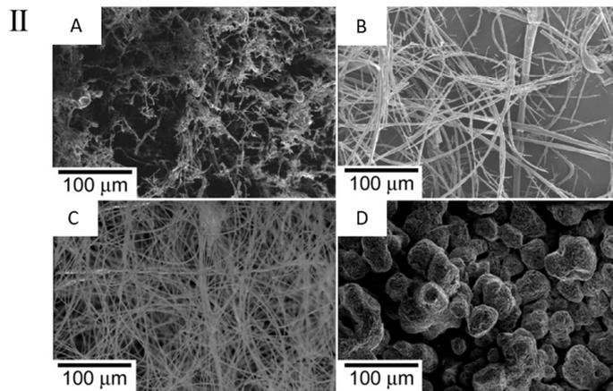
**Figure 5.** Change in morphology of electrospun Ca-containing  $\text{SiO}_2$  bioactive glass with the evolution in solution's viscosity resulting from solvent evaporation. SEM images (II) are named after the A to D domains of graph I, which gives viscosity values of electrospun solutions. Reproduced from [62]
