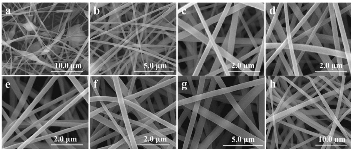
**Figure 6.** SEM images of silica fibres electrospun from a polymer-free solution. Viscosity values of the sol are a) 65 mPa.s, b) 102 mPa.s, c) 110 mPa.s, d) 125 mPa.s, e) 145 mPa.s, f) 198 mPa.s, g) 398 mPa.s and h) 981 mPa.s. Reproduced from [93]
