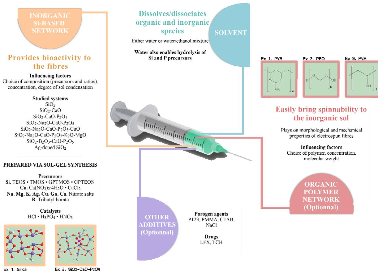
Figure 2. Considerations for the preparation of spinnable Si-based bioceramics with adequate bioactive properties
