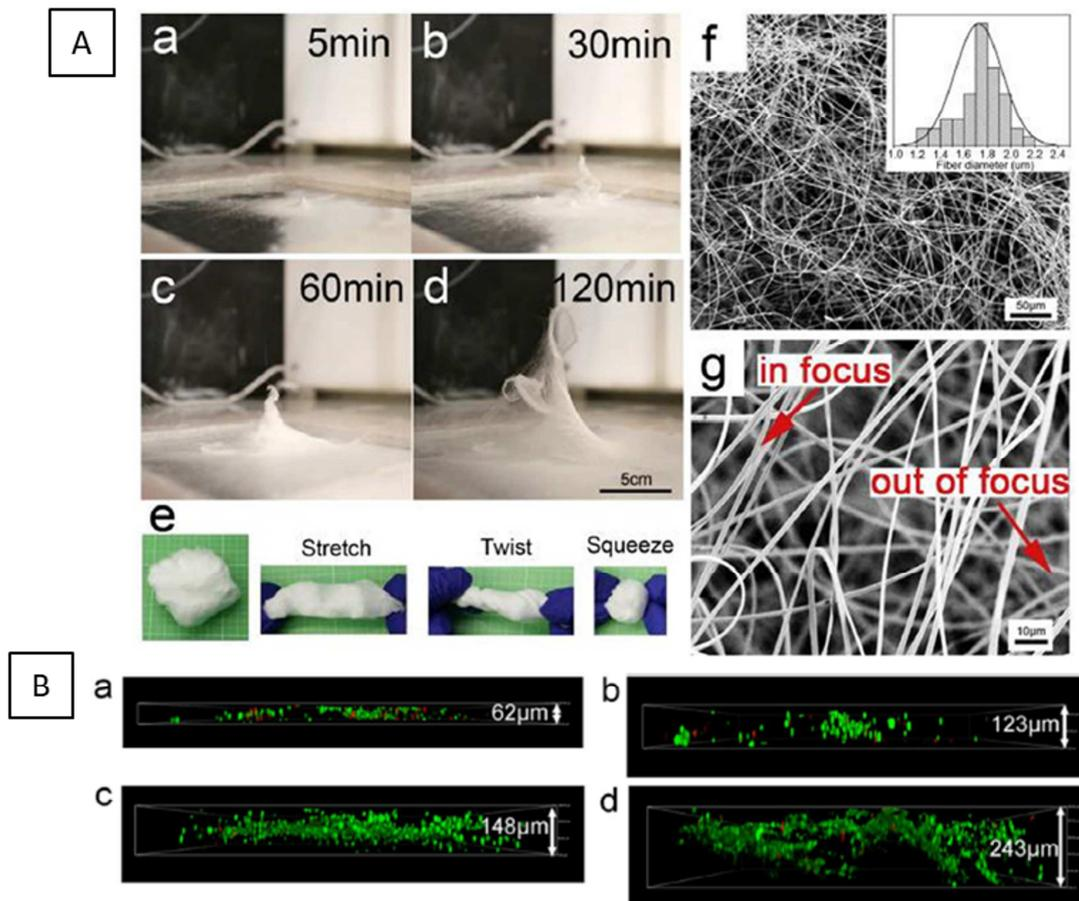
**Figure 9.** (A) (a-d) Electrospinning of TEOS/PVA sponge and 3D development with time; (e) deformation of silica sponge on a macroscopic level; (f-g) SEM images of the resulting fibres, with a fibre diameter distribution histogram as an insert in (f). (B) Confocal images of live/dead assay, showing the penetration depth of cells cultured on (a,c) silica membranes for 3 and 10 days respectively, and on (b,d) silica sponges for 3 and 10 days respectively. Reproduced from [50]
