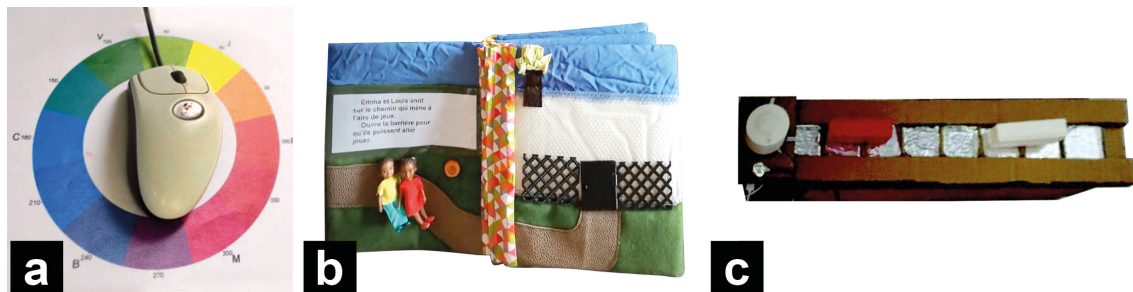
Fig. 6. Examples of interactive projects developed during hackathons: [a] a simple sensory substitution device, replacing colors with non-speech sounds; [b] spread from a sewn interactive book including small objects and recorded sounds; [c] a timeline made of cardboard and aluminium foil controlled by a Bare Conductive controller for exploring historical events and periods represented as 3D printed blocks, with spoken description of different complexity (changed using the knob).
