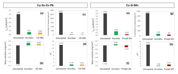
**Figure 3:** Assessment of the protectiveness of the selected coatings FA-MS (traditional bronze) and PropS-SH (modern bronze) compared to uncoated samples and Incralac coated samples: (a, e) Corrosion current density ( $i_{cor}$ ); (b, f) Mass variation induced by 10 days of ToW of Dropping test; (c, g) Cumulative Cu release in the weathering solutions during at the end of the artificial ageing; (d, h) Colour variation ( $\Delta E^*$ ) due to ageing.
