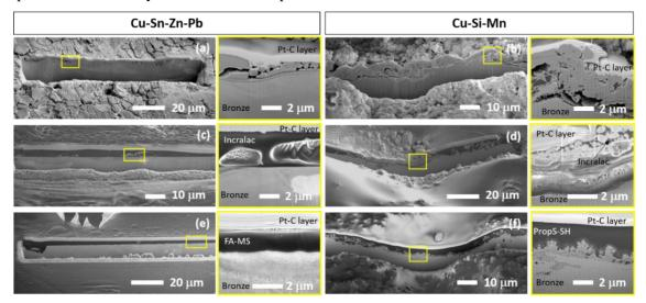
**Figure 4:** Observation of FIB cross-sections of uncoated and coated patinated Cu-Sn-Zn-Pb (left) and Cu-Si-Mn (right) after accelerated ageing by Dropping test: (a, b) uncoated patinated substrates; (c, d) Incralac; (e) FA-MS; (f) PropS-SH. Inlays of the FIB cross-sections at higher magnification are reported in yellow boxes.
