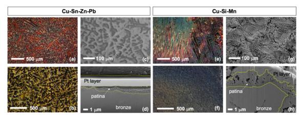
**Figure 2:** Microstructural observation of patinated bronze substrates before coating application (Cu-Sn-Zn-Pb and Cu-Si-Mn, respectively): (a, e) dendritic structure of bronze alloys; (b, f) patinated surfaces by optical microscope; (c, g) patinated surface morphologies observed by SEM; (d, h) representative FIB cross-sections of the patinated bronze substrates.
