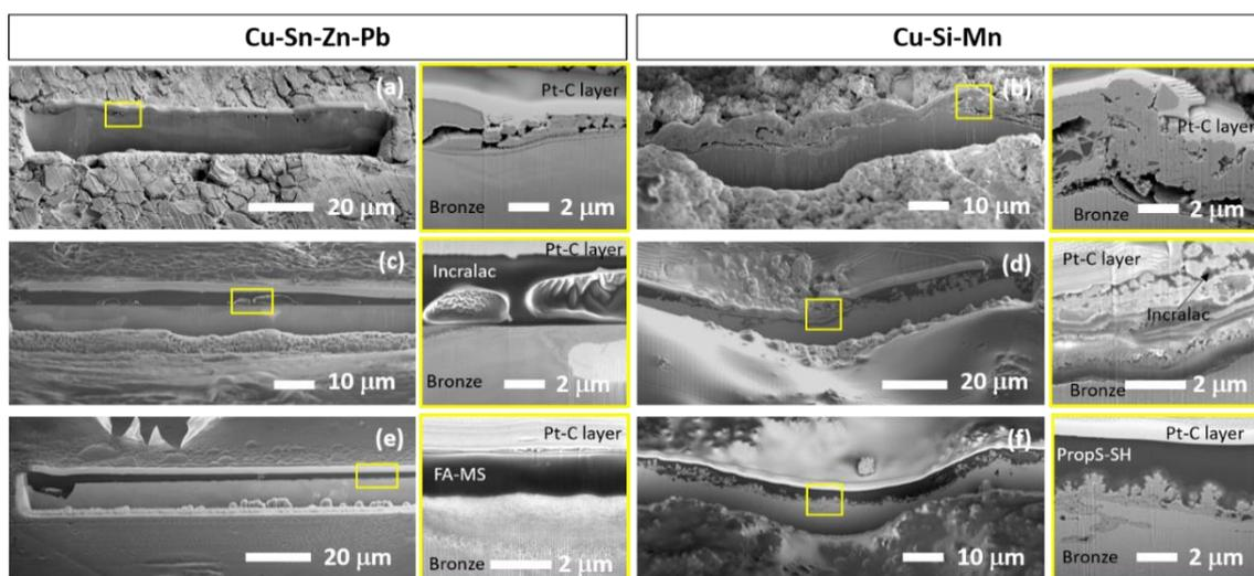
**Figure 4:** Observation of FIB cross-sections of uncoated and coated patinated Cu-Sn-Zn-Pb (left) and Cu-Si-Mn (right) after accelerated ageing by Dropping test: (a, b) uncoated patinated substrates; (c, d) Incralac; (e) FA-MS; (f) PropS-SH. Inlays of the FIB cross-sections at higher magnification are reported in yellow boxes.
