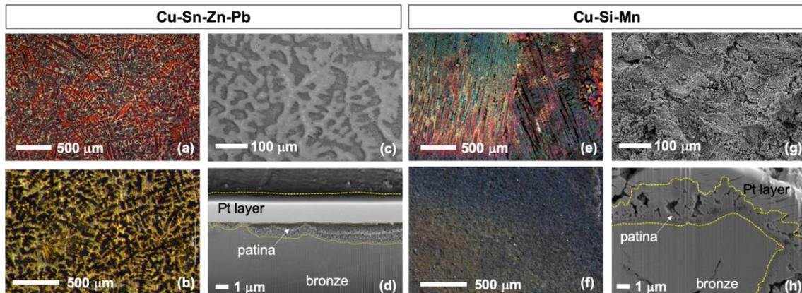
**Figure 2:** Microstructural observation of patinated bronze substrates before coating application (Cu-Sn-Zn-Pb and Cu-Si-Mn, respectively): (a, e) dendritic structure of bronze alloys; (b, f) patinated surfaces by optical microscope; (c, g) patinated surface morphologies observed by SEM; (d, h) representative FIB cross-sections of the patinated bronze substrates.
