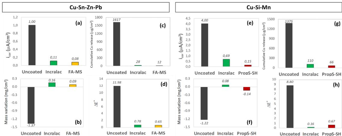
**Figure 3:** Assessment of the protectiveness of the selected coatings FA-MS (traditional bronze) and PropS-SH (modern bronze) compared to uncoated samples and Incralac coated samples: (a, e) Corrosion current density ( $i_{cor}$ ); (b, f) Mass variation induced by 10 days of ToW of Dropping test; (c, g) Cumulative Cu release in the weathering solutions during at the end of the artificial ageing; (d, h) Colour variation ( $\Delta E^*$ ) due to ageing.
