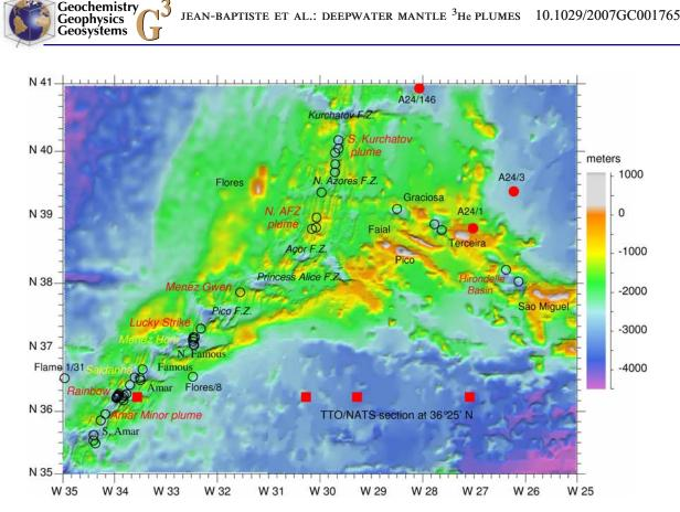
**Figure 1.** Location map of the MAR and of the Azores Archipelago. The open black circles represent the oceanographic stations occupied during the present survey. The red squares and dots are the "background" stations from the TTO/NATS section (1981) at 36.25°N and from the WOCE/A24 cruise (1997), respectively.
