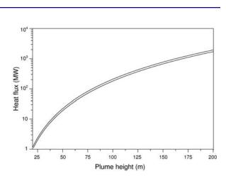
**Figure 11.** Heat output versus plume height calculated by the plume model for the north AFZ plume.
