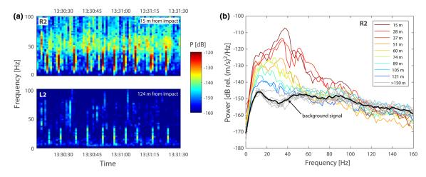
Figure 4. (a) Spectrograms of a series of 10 impacts that were performed at 15 m from R2 (top) and 124 m from L2 (bottom). (b) eismic power with distance from rock impact observed with geophone R2; the spectrograms at the time of the impact in panel (a) are represented as a line in panel (b).
