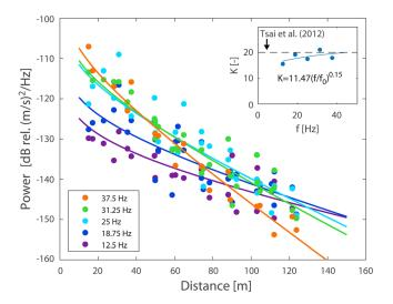
**Figure 5.** Seismic power decay with distance per frequency following the expression of the Green's function (equation 4). The inset shows the quality factor K derived from fitting normalized power based on the Green's function (see Supporting Information S2).
