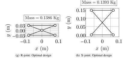
Figure 16: Specification B: Feasible design space, variation of joint mass, stiffness bounds and schematic of the optimal design corresponding to minimum mass, for both R-joint and X-joint, when  $F_{\rm max}=100$  N,  $\theta_{\rm rm}=\theta_{\rm xm}=0.7$  radians ( $\approx 40^{\circ}$ ),  $\underline{K}=10$  Nm/rad.
