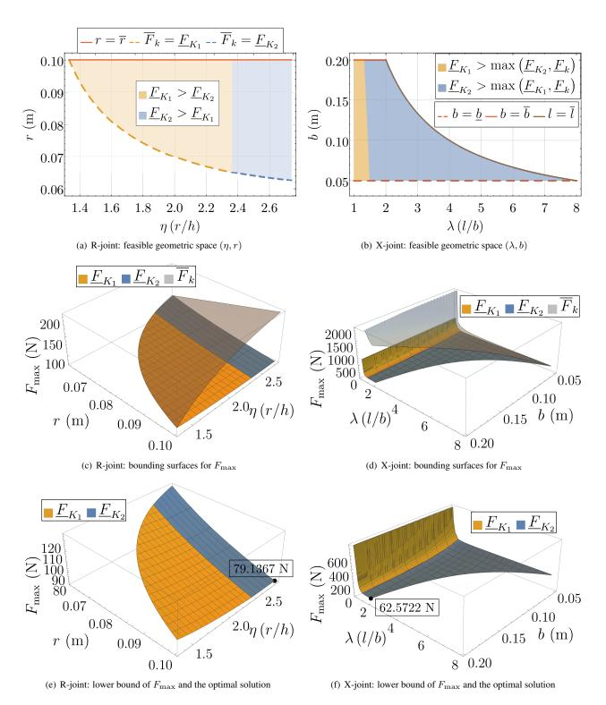
Figure 8: Specification B: Feasible geometric space and bounding surfaces of  $F_{\rm max}$  for both R-joint and X-joint, when  $\theta_{\rm rm}=\theta_{\rm xm}=0.7$  radians ( $\approx 40^{\circ}$ ),  $\underline{K}=10$  Nm/rad.
