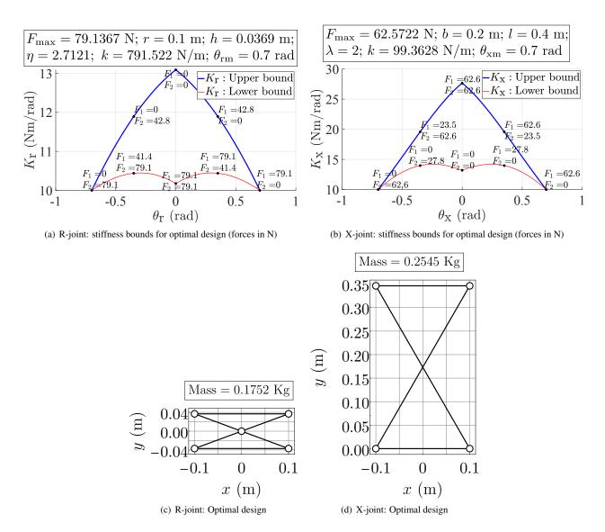
Figure 9: Specification B: Stiffness bounds and schematics of the optimal design corresponding to minimum  $F_{\rm max}$ , for both R-joint and X-joint, when  $\theta_{\rm rm}=\theta_{\rm xm}=0.7$  radians ( $\approx 40^{\circ}$ ),  $\underline{K}=10$  Nm/rad.
