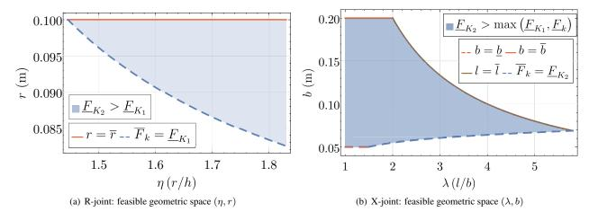
Figure 10: Specification C: Feasible geometric space for both R-joint and X-joint, when  $\theta_{rm}=\theta_{xm}=1.0$  radian ( $\approx 58^{\circ}$ ),  $\underline{K}=10$  Nm/rad.
