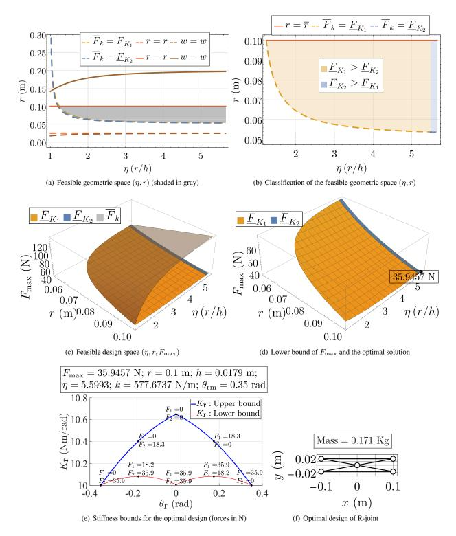
Figure 5: Specification A: Feasible geometric and design spaces, stiffness bounds and schematic of the optimal design minimizing the maximal actuation force for the R-joint, when  $\theta_{\rm rm}=0.35$  radians ( $\approx 20^{\circ}$ ),  $\underline{K}=10$  Nm/rad.
