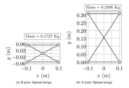
Figure 18: Specification C: Schematic of the optimal design corresponding to minimum mass, for both R-joint and X-joint, when  $F_{\rm max}=190$  N,  $\theta_{\rm rm}=\theta_{\rm xm}=1$  radian ( $\approx58^{\circ}$ ),  $\underline{K}=10$  Nm/rad.
