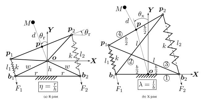
Figure 1: Schematics of the joints under study: R-joint (left) and X-joint (right).
