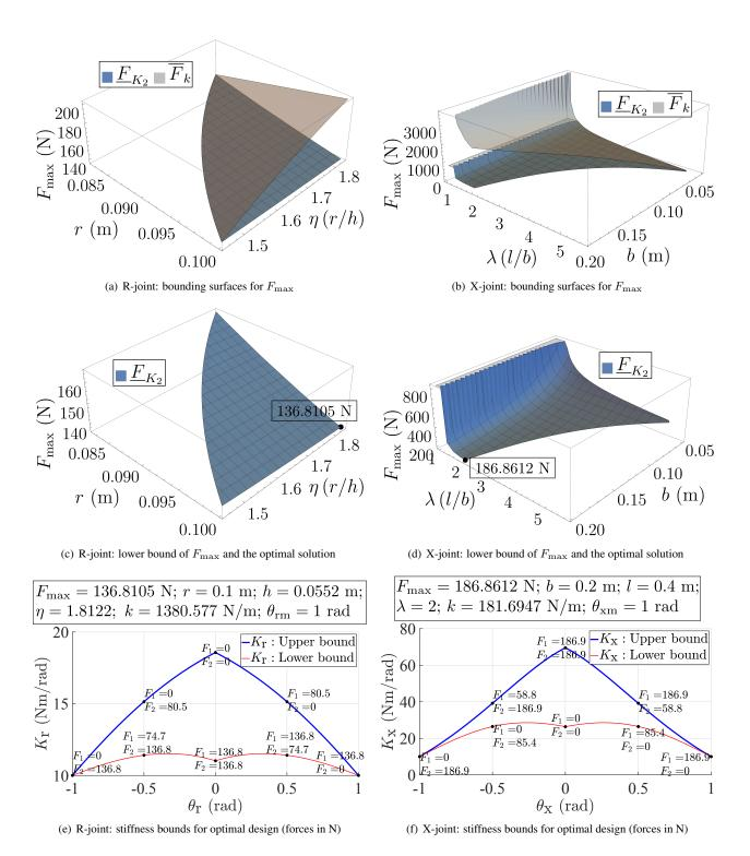
Figure 11: Specification C: Bounding surfaces of  $F_{\rm max}$ , stiffness bounds of the optimal design corresponding to minimum  $F_{\rm max}$ , for both R-joint and X-joint, when  $\theta_{\rm rm}=\theta_{\rm xm}=1.0$  radian ( $\approx 58^{\circ}$ ),  $\underline{K}=10$  Nm/rad.
