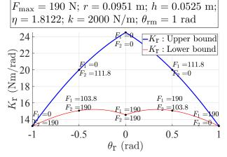
(e) R-joint: stiffness bounds for optimal design (forces in N)
