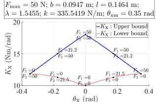
(f) X-joint: stiffness bounds for optimal design (forces in N)  $\,$
