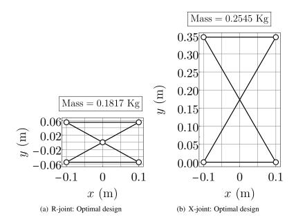
Figure 12: Specification C: Schematic of the optimal design corresponding to minimum  $F_{\rm max}$  for both R-joint and X-joint, when  $\theta_{\rm rm}=\theta_{\rm xm}=1.0$  radian ( $\approx 58^{\circ}$ ),  $\underline{K}=10$  Nm/rad.
