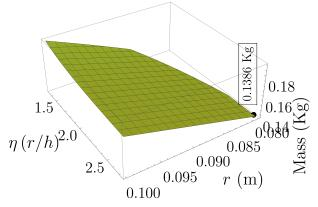
(c) R-joint: variation of mass inside the feasible design space and the minimum mass solution
