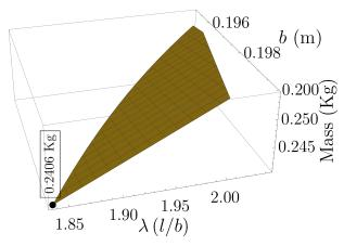
(d) X-joint: variation of mass inside the feasible design space and the minimum mass solution
