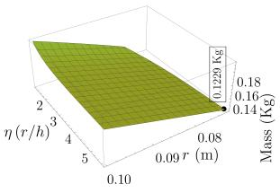
(c) R-joint: variation of mass inside the feasible design space and the minimum mass solution
