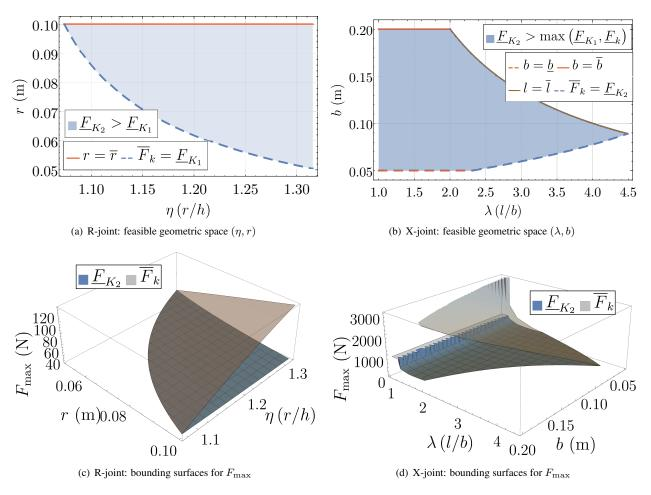
Figure 13: Specification D: Feasible geometric space and bounding surfaces for  $F_{\rm max}$  for both R-joint and X-joint, when  $\theta_{\rm rm}=\theta_{\rm xm}=1.3$  radians ( $\approx75^{\circ}$ ),  $\underline{K}=1$  Nm/rad.
