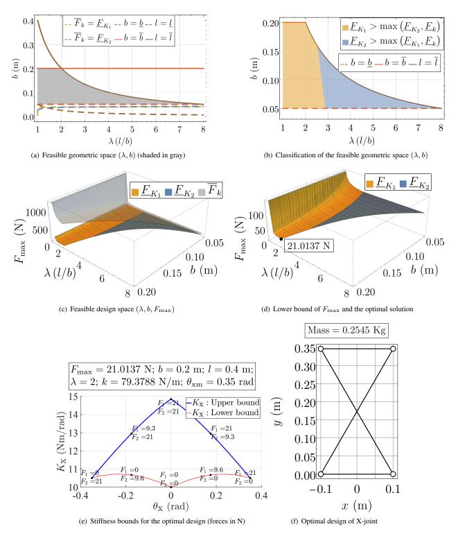
Figure 7: Specification A: Feasible geometric and design spaces, stiffness bounds and schematic of the optimal design minimizing the maximal actuation force for the X-joint, when  $\theta_{xm}=0.35$  radians ( $\approx 20^{\circ}$ ),  $\underline{K}=10$  Nm/rad.
