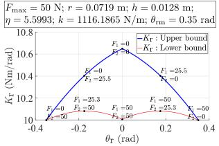
(e) R-joint: stiffness bounds for optimal design (forces in N)  $\,$
