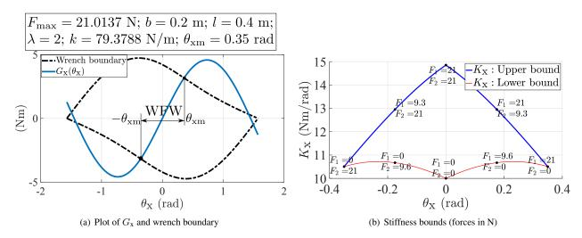
Figure 3: WFW (left) and stiffness bounds (right) for the X-joint.
