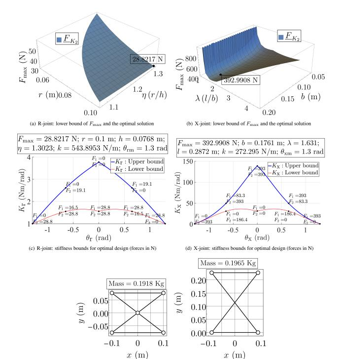
Figure 14: Specification D: Lower bounding surface for  $F_{\rm max}$ , stiffness bounds and schematic of the optimal design corresponding to minimum  $F_{\rm max}$ , for both R-joint and X-joint, when  $\theta_{\rm rm}=\theta_{\rm xm}=1.3$  radians ( $\approx75^{\circ}$ ),  $\underline{K}=1$  Nm/rad.
