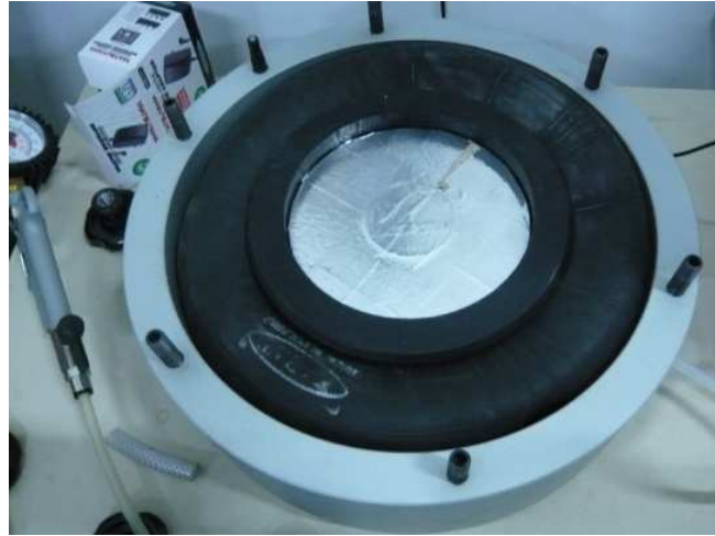
Fig. 1. Permeability cell accommodating the mortar coated with adhesive aluminum foil except at the micro-crack (pressure arrival side), the other side having undergone treatment by bioprecipitation was not covered with adhesive aluminum.
