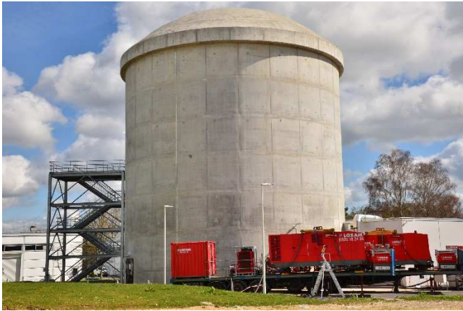
Fig. 2. A- VeRCORs: replica at 1/3 scale of a nuclear reactor enclosure; B- Sectional view
