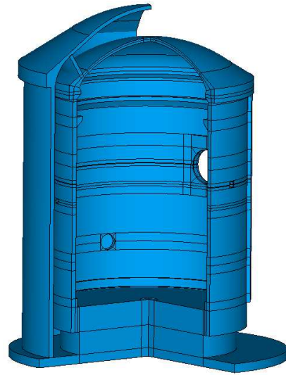
Fig. 2. A- VeRCORs: replica at 1/3 scale of a nuclear reactor enclosure; B- Sectional view
