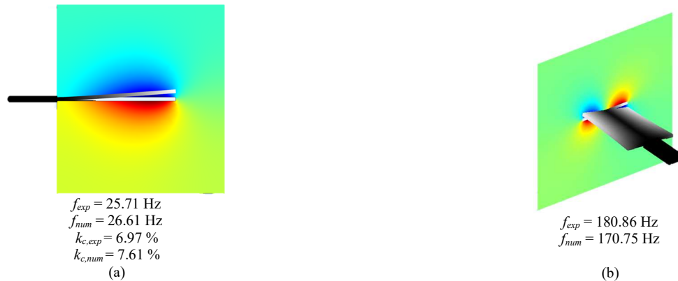
Fig. 11. Numerical mode shapes for still water with their associated natural frequencies and coupling factors compared to experimental results for (a) the first bending mode and (b) the first torsional mode. The colormap represents the pressure field within the fluid, while the gray shades represent the displacement field on the structure, from the numerical simulations.
