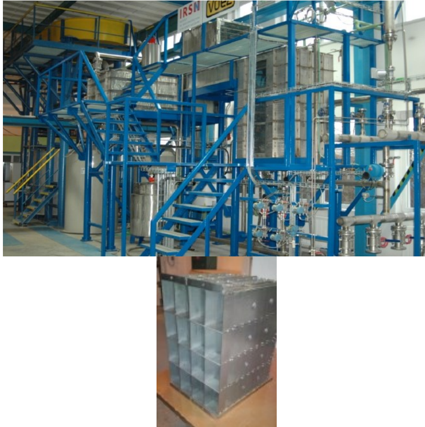
Figure 2 – VIKTORIA loop facility and view of the strainer mock-up.
