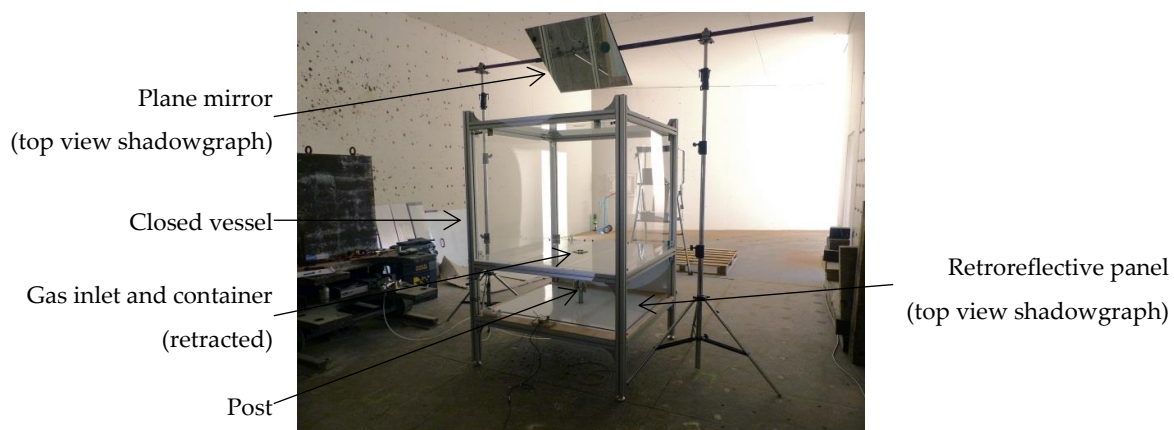
Figure 1. Global view of the experimental setup. The retro-reflective back panel was removed when the picture was taken.
