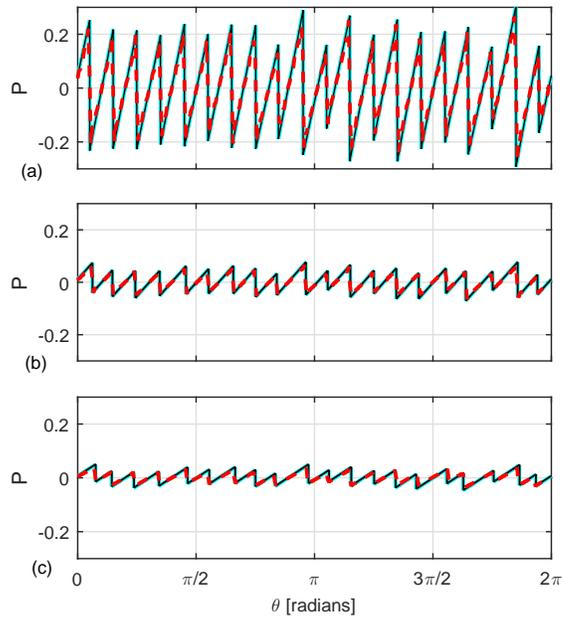
**Fig. 9** Comparison between numerical results from the TDNS, FDNS and 1DNP-TFD codes. Simulation of irregular sawtooth pressure waveform  $\underline{IR}_2$  in a rigid cylindrical intake duct: (a)  $z/D = 0$ , (b)  $z/D = 0.25$ , and (c)  $z/D = 0.5$ . Key: Blue line—TDNS; Red dashed line—FDNS; Black line—1DNP-TFD.
