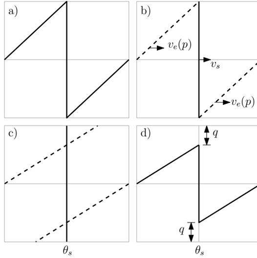
**Fig. 2** Illustration of the propagation and decay of a single N-wave, with mid-point pressure equal to the reference (mean) pressure. In this moving reference frame, the position of the shock,  $\theta_s$ , does not vary, but the shock amplitude is attenuated at its high- and low-pressure sides (shown by  $q$ ).
