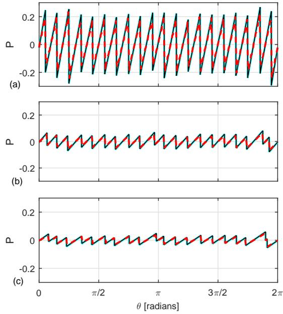
**Fig. 7** Comparison between numerical results from the TDNS, FDNS and 1DNP-TFD codes. Simulation of irregular sawtooth pressure waveform  $\underline{IR}_1$  in a rigid cylindrical intake duct: (a)  $z/D = 0$ , (b)  $z/D = 0.25$ , and (c)  $z/D = 0.5$ . Key: Blue line—TDNS; Red dashed line—FDNS; Black line—1DNP-TFD.
