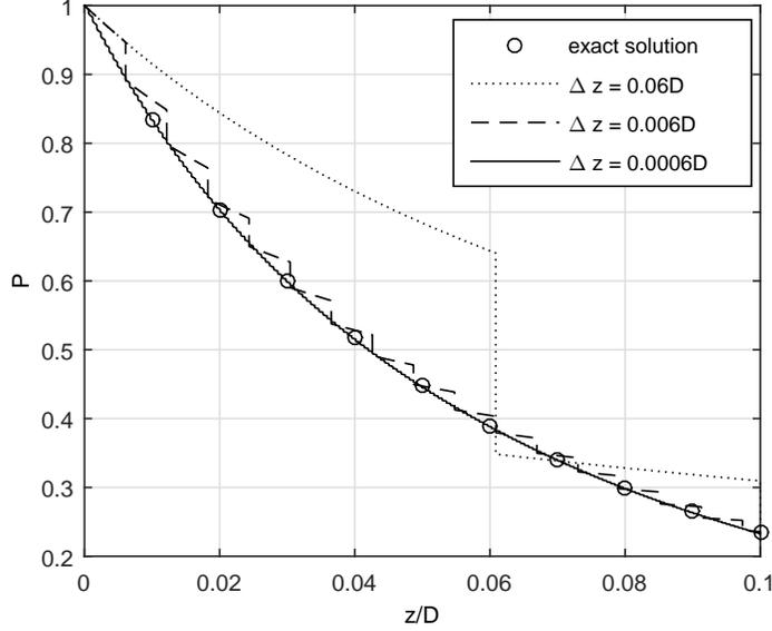
**Fig. 5 Amplitude of the BPF tone as a function of axial position for a regular sawtooth waveform in a lined duct. Example for a sawtooth with 20 shocks, initial shock strength  $s = 0.432$  and constant liner absorption rate.**
