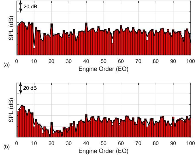
Fig. 13 Comparison between numerical results from the FDNS and 1DNP-TFD codes. EO frequency spectrum for irregular sawtooth  $\underline{IR}_1$  in a lined cylindrical intake duct: (a)  $z/D = 0.25$ , and (b)  $z/D = 0.5$ . Key: Red bars—FDNS; Black line—1DNP-TFD.
