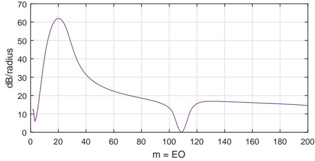
**Fig. 11 Linear decay rates for engine orders 1 to 100.**
