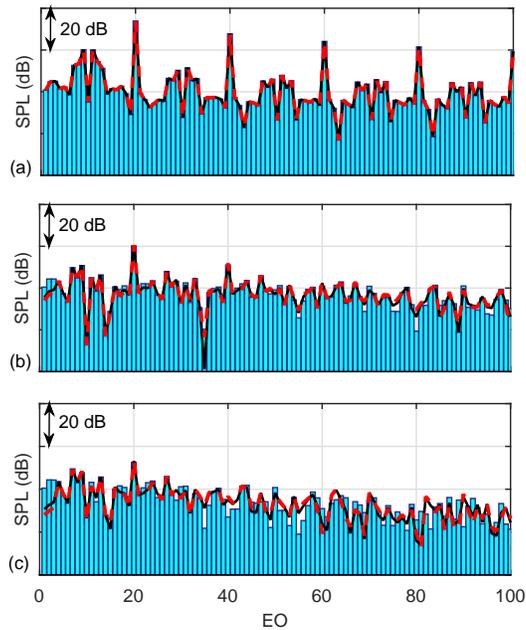
**Fig. 10** Comparison between numerical results from the TDNS, FDNS and 1DNP-TFD codes. EO frequency spectrum for irregular sawtooth  $\underline{IR}_2$  in a rigid cylindrical intake duct: (a)  $z/D = 0$ , (b)  $z/D = 0.25$ , and (c)  $z/D = 0.5$ . Key: Blue bars—TDNS; Red dashed line—FDNS; Black line—1DNP-TFD.
