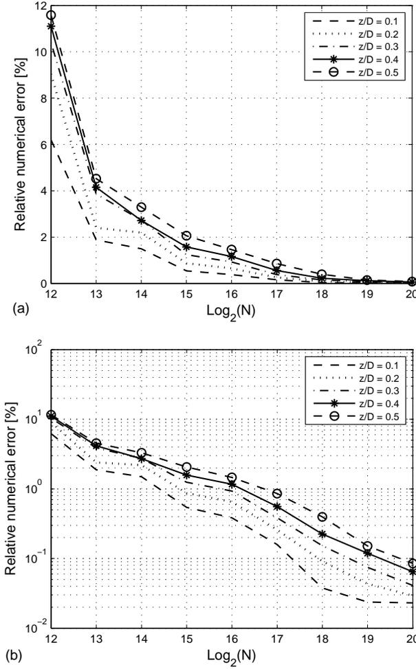
**Fig. 4** Relative numerical error shown on a linear scale (a) or logarithmic scale (b) for the propagation of a regular sawtooth in a rigid duct for various grid resolutions. Example for a sawtooth with 20 shocks and initial shock strength  $s = 0.432$ .
