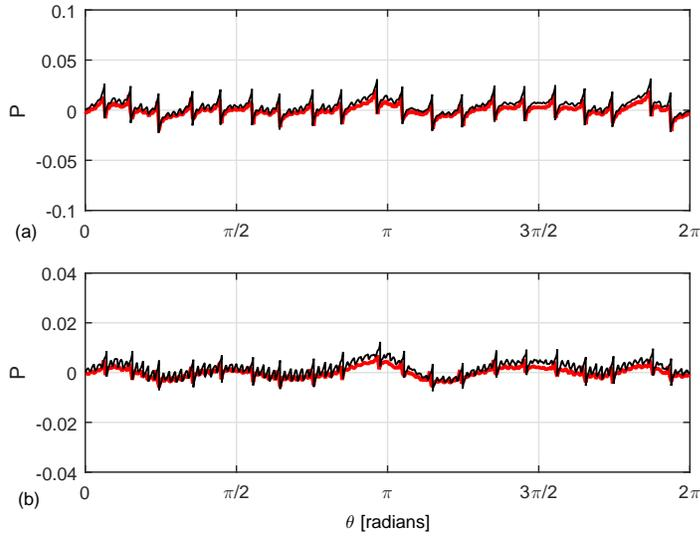
Fig. 12 Comparison between numerical results from the FDNS and 1DNP-TFD codes. Simulation of irregular sawtooth pressure waveform  $\underline{IR}_1$  in a lined cylindrical intake duct: (a)  $z/D = 0.25$ , and (b)  $z/D = 0.5$ . Key: Red line—FDNS; Black line—1DNP-TFD.
