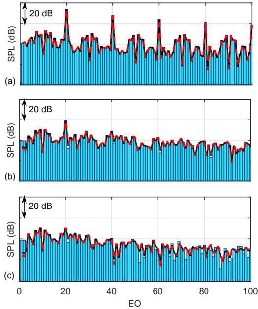
**Fig. 8** Comparison between numerical results from the TDNS, FDNS and 1DNP-TFD codes. EO frequency spectrum for irregular sawtooth  $\underline{IR}_1$  in a rigid cylindrical intake duct: (a)  $z/D = 0$ , (b)  $z/D = 0.25$ , and (c)  $z/D = 0.5$ . Key: Blue bars—TDNS; Red dashed line—FDNS; Black line—1DNP-TFD.
