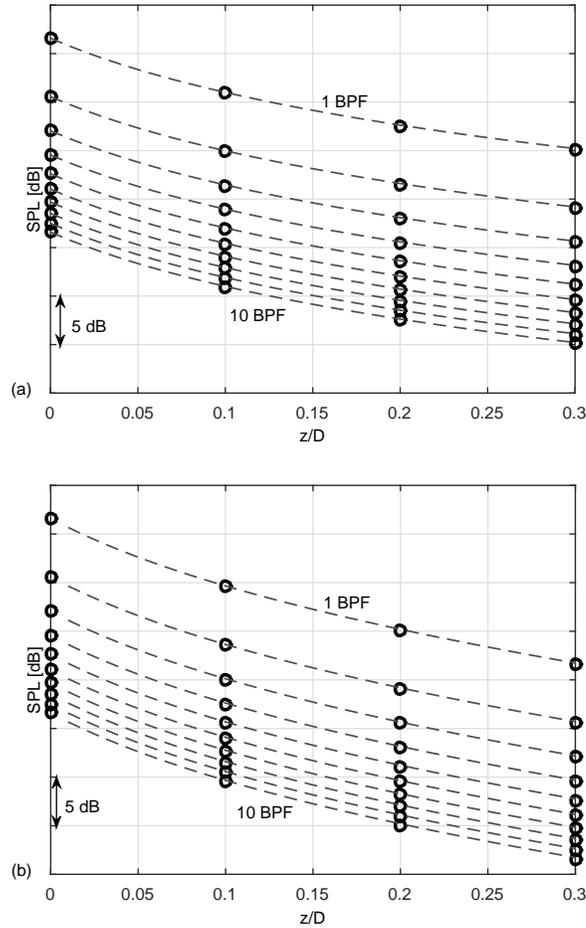
**Fig. 6** Comparison of the amplitudes of the first ten BPF harmonics for a regular sawtooth in a rigid duct (a) and a lined duct with a constant liner absorption rate (b). Key: Symbols—Numerical results; Dashed lines—Analytic solutions.
