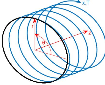
**Fig. 1** Illustration of the helical path traced out by the sawtooth waveform inside a cylindrical intake duct.
