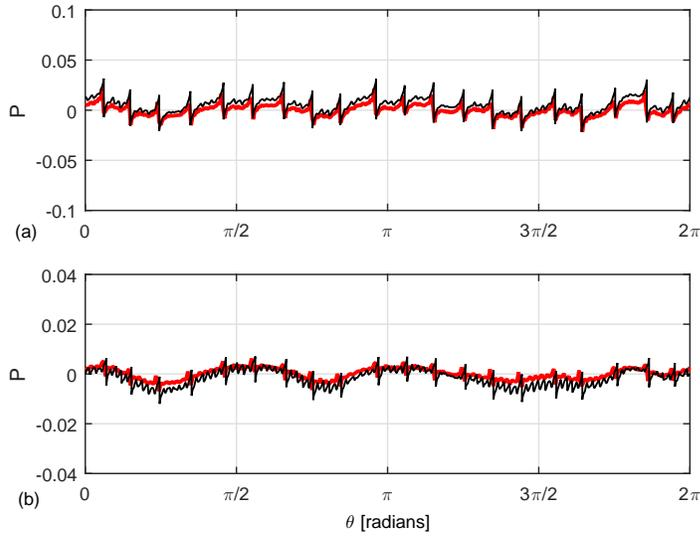
Fig. 14 Comparison between numerical results from the FDNS and 1DNP-TFD codes. Simulation of irregular sawtooth pressure waveform  $\underline{IR}_2$  in a lined cylindrical intake duct: (a)  $z/D = 0.25$ , and (b)  $z/D = 0.5$ . Key: Red line—FDNS; Black line—1DNP-TFD.
