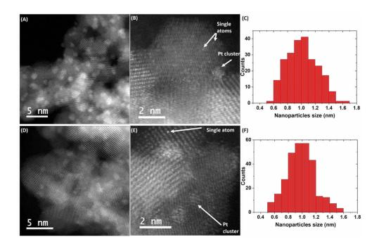
Figure 2. Representative HAADF-STEM images of the Pt/CeO<sub>2</sub> catalyst and the corresponding distribution of Pt particle sizes before (A-C) and after CO oxidation under wet conditions (D-E).
