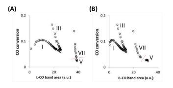
Figure 4. CO conversion plotted against the band area of  $Pt^0$ -bound (A) L-CO and (B) B-CO corresponding to periods I, III, V and VII as indicated in Figure 3.A.
