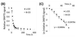
**Figure 7.** (A) DRIFTS spectra collected over the Pt/CeO<sub>2</sub> at 30 °C under 0.6 % water + 2 % O<sub>2</sub>/He at various times following the removal of CO. These data correspond to the region II in Figure 3.A. The band intensity of the linear L-CO and bridged B-CO species was then plotted as a function of time in (B) normal or (C) semi-logarithmic coordinates.
