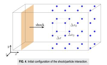
cloud is also initially structured according to a cubic particle shape. The load rate  $\tau_{\nu,0}$  of this cloud is also the ratio between the volume taken by the particles and the volume of the gas. The initial organization of the particles and the initial load rate are shown in Fig. 4. With such a cubic arrangement, the load rate is
