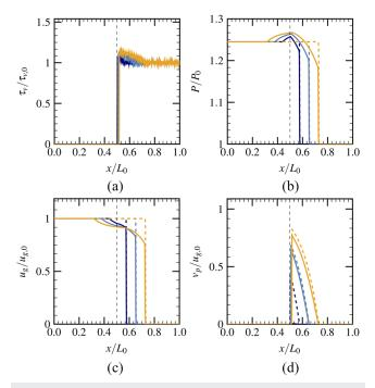
**FIG. 10**. Comparison one-way/two-way for different time instants. One-way on 0.2 ms (dark blue dashed line), 0.4 ms (blue dashed line), and 0.6 ms (orange dashed line) and two-way on 0.2 ms (dark blue solid line), on 0.4 ms (blue solid line), 0.6 ms (orange solid line);  $\tau_{v,0} = 5.2 \times 10^{-4}$ ,  $d_p = 10 \ \mu m$ ,  $\rho_p = 10^3 \ kg/m^3$ , original contact surface (black dashed line); (a) droplet volume fraction, (b) gas pressure, (c) gas velocity, and (d) droplet velocity.
