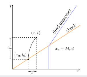
**FIG. 1**. Space-time diagram (x, t) of the considered system with  $x_s$  the shock position, x' the distance covered by a particle located initially at  $x_0$ , and t' the duration of the interaction of the particle with the shock.
