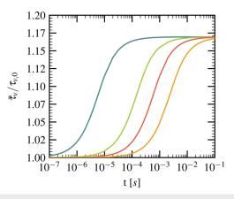
**FIG. 3.** Mean load rate evolutions for particles of different  $\tau_p$  in air:  $\tau_p = 3 \times 10^{-6}$  s (blue solid line),  $\tau_p = 7.5 \times 10^{-5}$  s (green solid line),  $\tau_p = 3 \times 10^{-4}$  s (red solid line),  $\tau_p = 1.2 \times 10^{-3}$  s (orange solid line),  $\rho_p = 10^3$  kg/m<sup>3</sup>,  $M_s = 1.1$ , and  $u_g = 55.19$  m/s.
