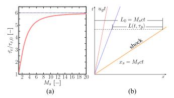
**FIG. 2.** Cloud density as a function of the Mach number and the length of cloud in the post-shock area. (a) Evolution of  $\overline{\tau_v}/\tau_{v,0}$  as a function of  $M_{s_i}$ , the dashed blue line represents the asymptotic limit given by  $(\gamma + 1)/(\gamma - 1)$  with  $\gamma = 1.4$ . (b) Space–time diagram showing the cloud length pre- and post-shock.
