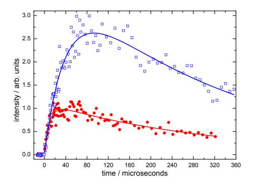
Figure 1 H-atom formation curves recorded at 50 K for the  $C(^{1}D)$  + NO reaction using the  $H_{2}$  chemical tracer method. (Open blue squares) without NO,  $[H_{2}] = 1.2 \times 10^{14}$  cm<sup>-3</sup>; (solid red circles)  $[NO] = 8.9 \times 10^{14}$  cm<sup>-3</sup>,  $[H_{2}] = 1.2 \times 10^{14}$  cm<sup>-3</sup>. Solid blue and red lines represent biexponential fits to the individual datapoints using expression (1).
