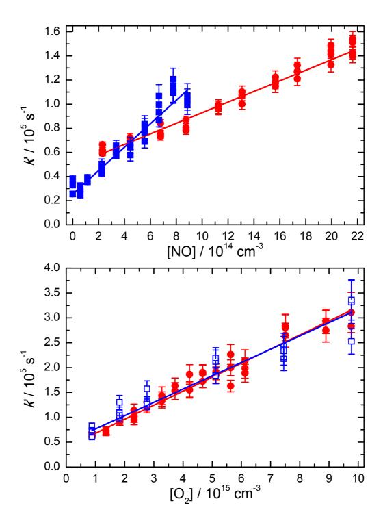
**Figure 2** Pseudo-first-order rate constants as a function of coreagent concentration. Top panel: the  $C(^{1}D)$  + NO reaction; (solid blue squares) 50 K; (solid red circles) 296 K. Bottom panel:
