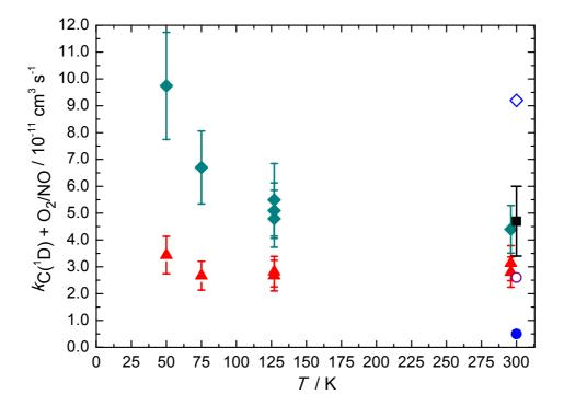
**Figure 3** Rate constants for  $C(^{1}D)$  reactions as a function of temperature.  $C(^{1}D)$  + NO: (solid green diamonds) this work; (solid black square) Husain and Kirsch [32]; (open blue diamond) Braun et al. [35].  $C(^{1}D)$  +  $O_{2}$ : (solid red triangles) this work; (open purple circle) Husain and Kirsch [32]; (solid blue circle) Braun et al [35].
