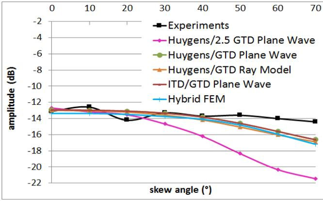
Fig. 7. Echo amplitude diffracted by the top tip.
