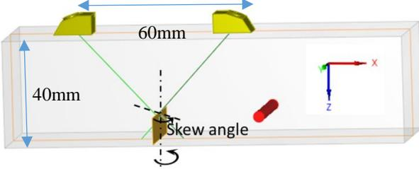
Fig. 6. TOFD inspection used for experimental validation.
