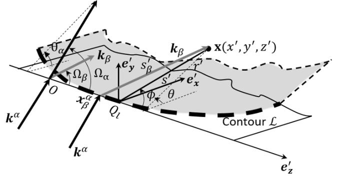
Fig. 1. A plane wave with the propagation vector  $\mathbf{k}^\alpha$  incident on a stress-free crack (in gray) of contour  $\mathcal{L}$ . Thick black arrow – direction of the incident wave; thick gray arrow - direction of the wave scattered by the half-plane tangent to the crack at the diffraction point  $Q_l$ .
