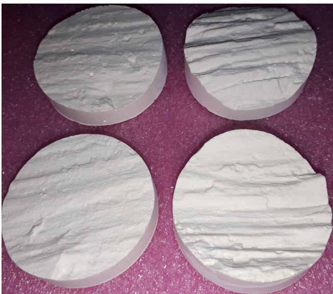
FIG. 4. Plaster faults made using the 3D-printed moulds (i.e., an example of which is shown in Fig. 4). Left: S_m (top) and its complementary surface (bottom). Right: S_{mm} (top) and its complementary surface (bottom). The samples have a diameter of 40 mm. One can appreciate that the fault at the millimeter scale ( S_{mm} ) shows a higher roughness aspect than at the meter scale ( S_m ).
