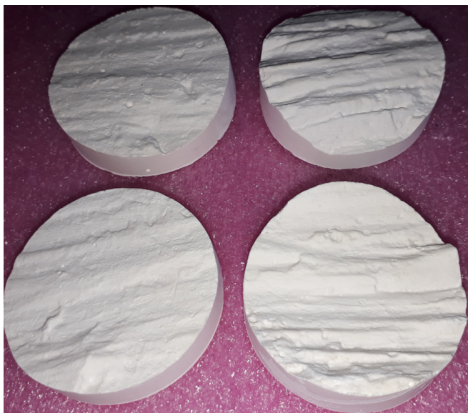
FIG. 4. Plaster faults made using the 3D-printed moulds (i.e., an example of which is shown in Fig. 4). Left: S_m (top) and its complementary surface (bottom). Right: S_{mm} (top) and its complementary surface (bottom). The samples have a diameter of 40 mm. One can appreciate that the fault at the millimeter scale ( S_{mm} ) shows a higher roughness aspect than at the meter scale ( S_m ).
