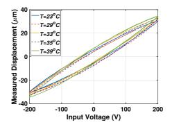
**FIGURE 2**. Measured voltage-to-displacement hysteresis loops of the piezotube actuator by applying a harmonic input voltage of  $u(t) = 200 \sin(2\pi \text{ ft})$  V with the excitation frequency f = 0.1 Hz under different levels of environmental temperature of T = 23°C, 29°C, 33°C, 35°C, and 39°C.
