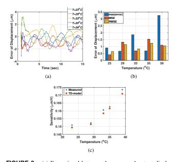
**FIGURE 8.** (a) Error signal between the measured output displacement and the proposed hysteresis model output using threshold number n = 9 at different environmental temperatures, (b) Maximum error, Mean square error (MSE) and Root mean square error (RMSE) for the measured output displacement and the proposed model hysteresis output, and (c) comparison of the sensitivity of the measured data and the proposed hysteresis model.
