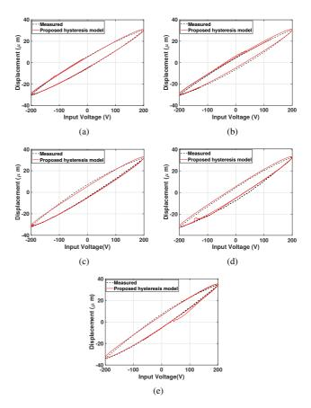
**FIGURE 7**. Comparison between the measured voltage-displacement hysteresis loop and the proposed hysteresis model voltage-displacement hysteresis loop using threshold number of n = 9 at different environmental temperatures: (a)  $T = 23^{\circ}C$ , (b)  $T = 29^{\circ}C$ , (c)  $T = 33^{\circ}C$ , (d)  $T = 35^{\circ}C$ , and (e)  $T = 39^{\circ}C$ .
