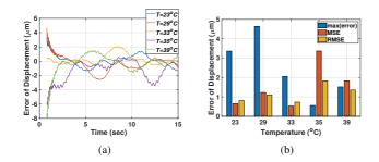
**FIGURE 9**. (a) Error signal between the measured output displacement and the proposed hysteresis model output using threshold number n = 5 at different environmental temperatures, and (b) Maximum error, Mean square error (MSE) and Root mean square error (RMSE) for the measured output displacement and the proposed hysteresis output,
