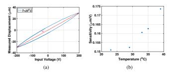
**FIGURE 3**. (a) The slope of the best linear model of hysteresis loop, and (b) The calculated sensitivity of the piezotube actuator under different levels of environmental temperature of  $T = 23^{\circ}C$ ,  $29^{\circ}C$ ,  $33^{\circ}C$ ,  $35^{\circ}C$ , and  $39^{\circ}C$ .
