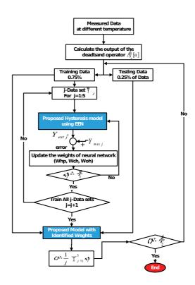
**FIGURE 5**. Flow chart of training algorithm for proposed hysteresis model.
