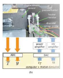
**FIGURE 1**. The experimental platform: (a) PT230.94 piezotube actuator, and (b) PT230.94 piezotube actuator with the displacement sensor, heater resistor, thermal sensor probe, power amplif er, and dSpace card.
