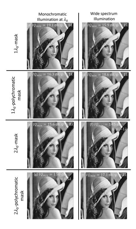
Fig 14 Restored images for different illuminations (column) and different masks (rows). In each case, the image corresponding to the worse image quality over the DoF range is represented. The value of defocus parameter  $\psi$  for which is image is obtained, and the corresponding value of  $IQ_{min}$  are given on each image.
