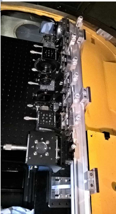
Shack-Hartmann wavefront sensor at the telescope
