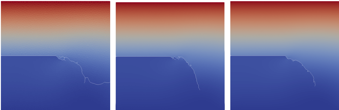
Figure 15: Single-edge notched shear test: u_x in colors and crack path in white, u_D = 0.2\text{mm} . Left: coarse mesh. Middle: fine mesh. Right: finest mesh.
