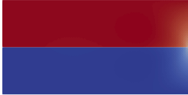
Figure 12: Opening mode: u_y in colors and crack path in white on a structured mesh.
