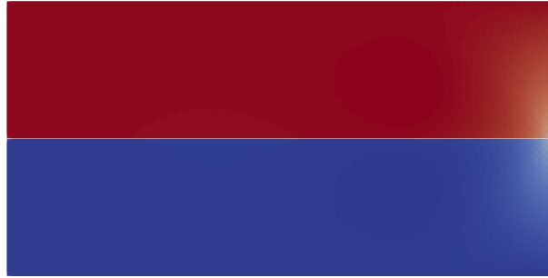
Figure 12: Opening mode: u_y in colors and crack path in white on a structured mesh, u_D = 2.5\text{mm} .
