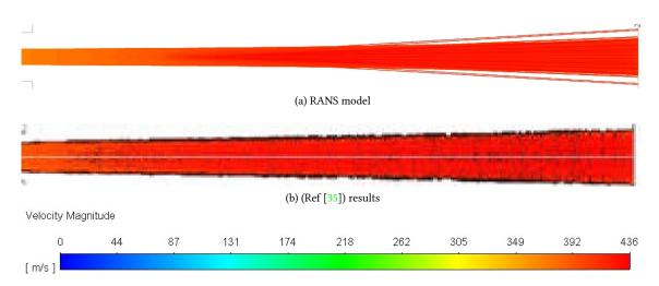
Figure 9: Particles track colored according to their velocity magnitude between the exit of the nozzle and the substrate for configuration B. The scale is 3/2
