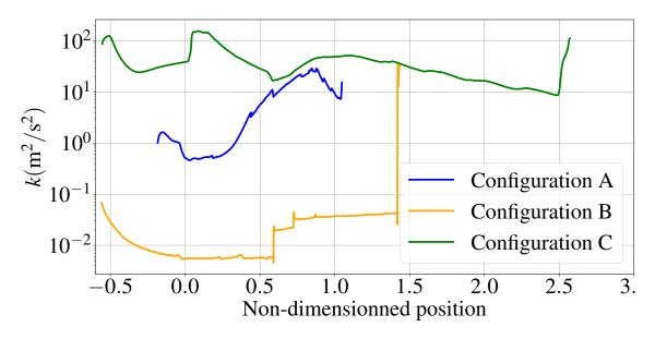
Figure 14: k as a function of the dimensionless position along the nozzle on the axis of symmetry from IDDES model on configurations A to C. The dimensionless position corresponds to the position divided by L. Dimensionless position 0 corresponds to the nozzle throat
