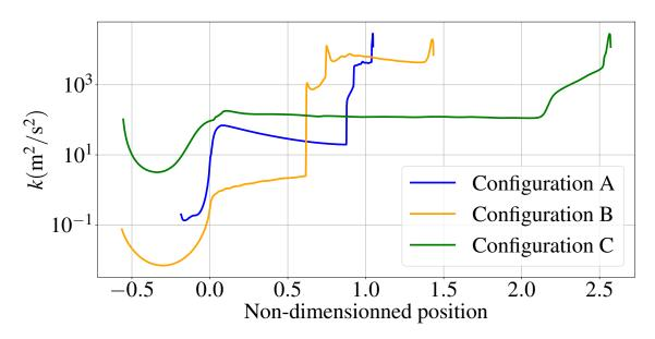
Figure 7: k as a function of the dimensionless position along the nozzle on the axis of symmetry from RANS model results on configurations A to C. The dimensionless position corresponds to the position divided by L. Dimensionless position 0 corresponds to the nozzle throat
