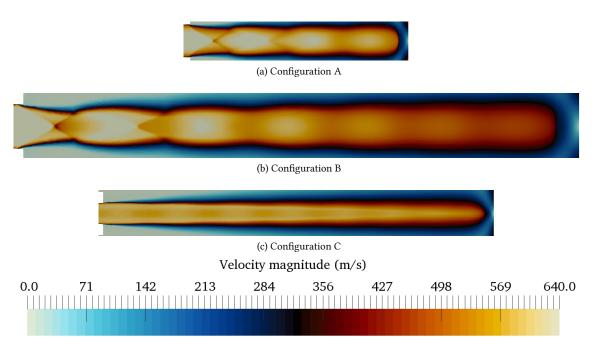
Figure 5: Velocity magnitude of the flow between the exit of the nozzle and the substrate for the configuration A to C. The scale is 3/2.
