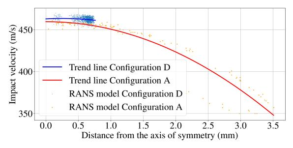
Figure 20: Particle impact velocity as a function of the distance from the axis of symmetry for configuration A and D with RANS model
