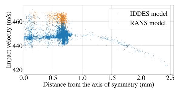
Figure 21: Particle impact velocity as a function of the distance from the axis of symmetry for configuration D for IDDES model and RANS model
