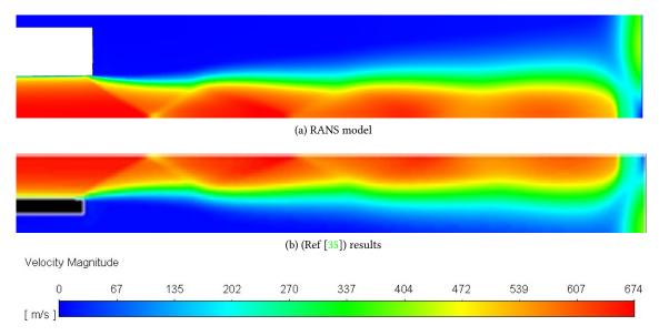
Figure 6: Velocity magnitude of the flow from the exit to the substrate for configuration A with RANS model comparing with the results in (Ref [35])
