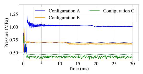
Figure 15: Pressure as a function of time at the intersection of the axis of symmetry and the substrate. The solid curves correspond to the IDDES model and the dotted lines correspond to the RANS value constant along time.
