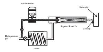
Figure 1: Diagram of a convergent-divergent channel De Laval (cf (Ref [1]))
