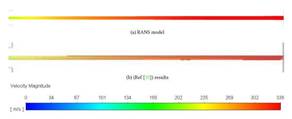
Figure 10: Particles track colored according to their velocity magnitude between the exit of the nozzle and the substrate for configuration C. The scale is 15/7
