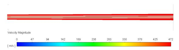
Figure 18: Particle tracks colored according to their velocity magnitude between the exit of the nozzle and the substrate for configuration D with RANS model. The scale is 15/4.
