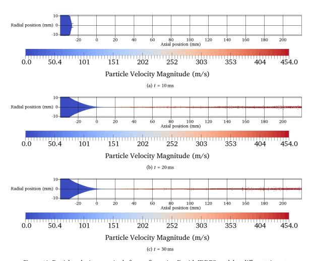
Figure 19: Particle velocity magnitude for configuration D with IDDES model at different time steps.
