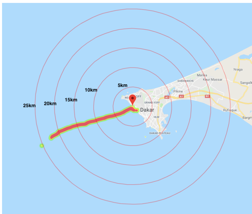
Figure 18: Received Signal with RSSI higher than -95dBm
