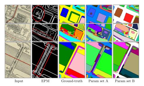
Fig. 4: Some failures and some success stories of the watershed segmentation. The parameter sets are A: h=3,  $\lambda = 250$ , and B: h=7,  $\lambda = 400$ . The first row shows the ability to recover weak boundaries. This sensitivity is not desirable in some cases as it leads the over-segmentation of the 2nd row. The third row suggests that the over-segmentation can be prevented by a stronger filtering but would also lead to a lower shape detection.
