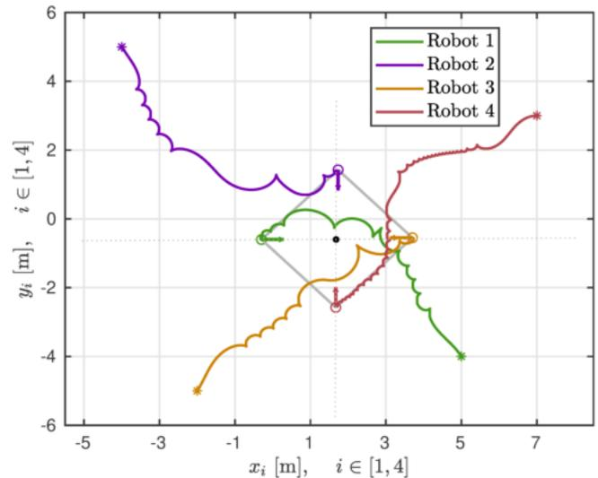
Fig. 3. Trajectories and formation of the network of mobile robots.
