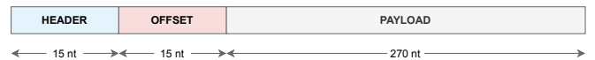
Fig. 2. General format of a Data Oligo. The header contains the information related to the type of oligo and DWT. The offset encodes the position of the data in the initial subband.
