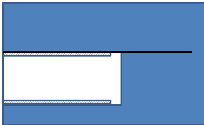
(c) horizontal pipes leaning on the concrete lining already built
