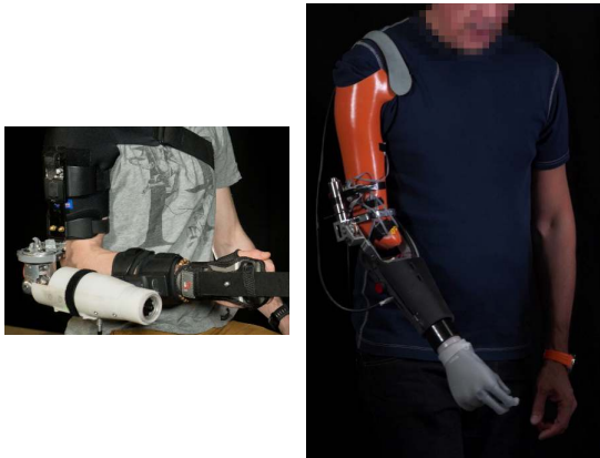
(a) Emulated elbow prosthesis prototype for able-bodied subjects (b) Prosthesis of the amputated subject
