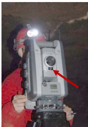
Figure 7: The Trimble VX™ spatial station is equipped with a 3 Megapixel built-in camera (just below the telescope of the instrument)
