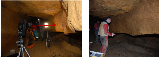
Figure 10. Recording of a clay panel with the Trimble VX™
