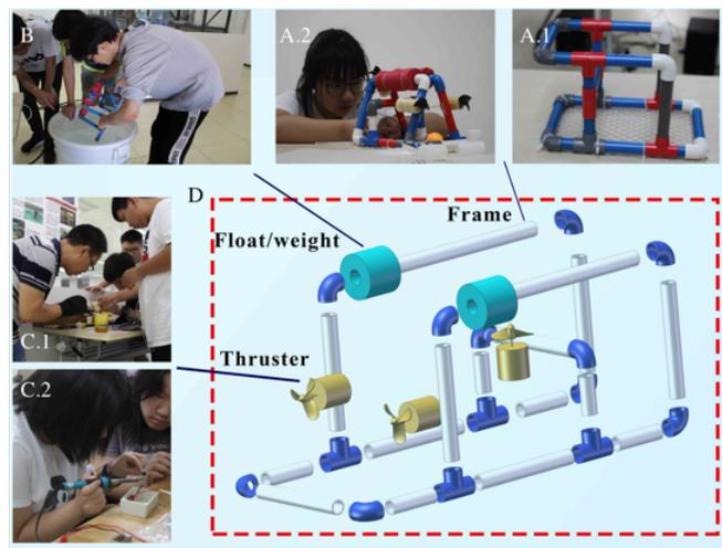
Fig. 4. Key educational components of the “Sea Perch” underwater robots. A.1 and A.2: Frame assembly for structural integrity; B: Floater placement for hydrostatics; C.1 and C.2: Motor waterproof and control box construction.
